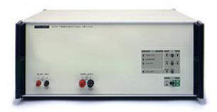
The 5220A Transconductance Amplifier lets you calibrate alternating or direct current meters and shunts and the current functions of digital multimeters that measure up to 20A. A known input voltage of 1 to 20 volts produces a known output current of 1 to 20A.
