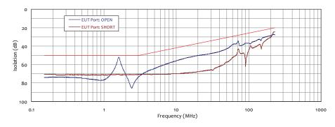
${\tt Data\ shown\ on\ above\ graphs\ is\ representative\ of\ a\ typical\ CDN\ M325E\ Coupling/Decoupling\ Network.}$
