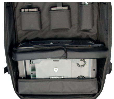
Fig. 9. Correct orientation of the SignalShark in the Backpack.
