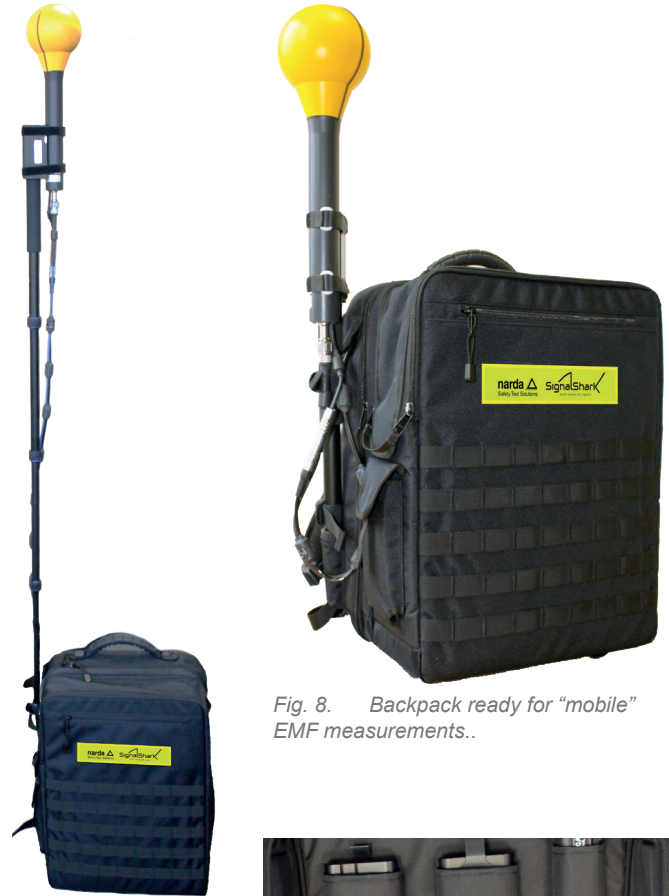
Fig. 7. Backpack in “tripod mode”.
