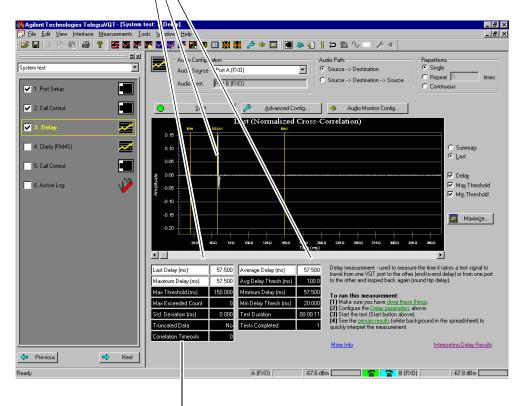
One very important parameter to look at when evaluating measurement results is the Correlate Timeout parameter. If this field is red, it is highly likely that measurement results are invalid. Correlation Timeouts can occur when excessive noise is present on the line or when the call is unexpectedly disconnected. In the example above, the measurement did not timeout.
