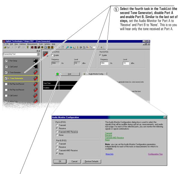
Start transmitting the tone from Port B. When you hear the tone, you will know that you have connectivity between Port B and Port A because of the way the Audio Monitor is configured.
