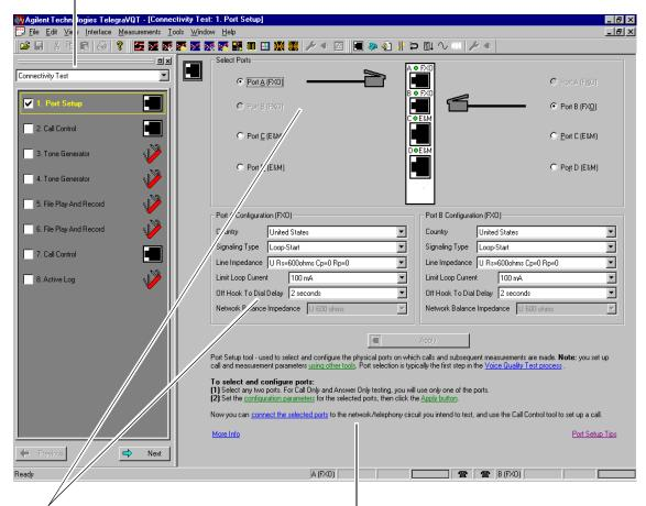
Notice that Ports A and B are selected (the FXO ports). Also note that you can configure the electrical characteristics of the ports. For this example, these selections and default configurations can be left as they are.
