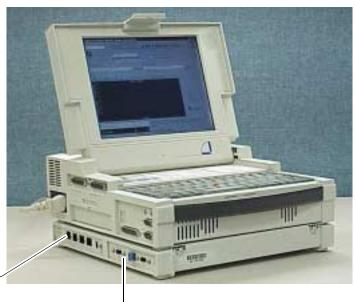
The analog signal acquisition ports are located on the left side of the chassis.
