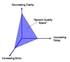
The relationships between clarity, delay, and echo can be quite complex as shown in the three dimensional figure above. If you think of voice quality as a single plotted point in the graph, you can see that voice quality improves as the point is plotted closer to the intersection of the three lines. In other words, as the distance between the voice quality "point" and the intersection increases, voice quality decreases.
