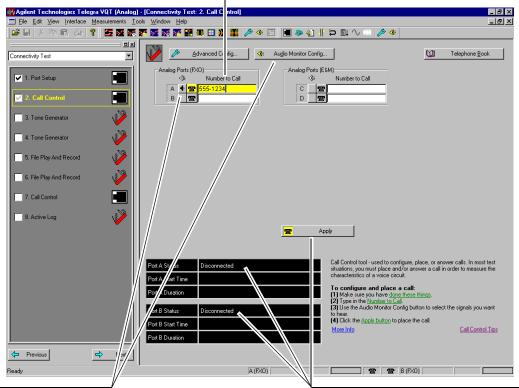
Select the port you want to monitor (in this case Port A). Then click the Audio Monitor Config button and set the parameter to 'Transmit AND Receive'. These two settings allow you to hear the dial tone, the DTMF dialing, and ringing.
