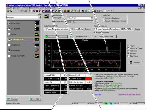
Notice that the Correlation Timeout parameter shows 'No'. This indicates that the Clarity measurement received the distorted test signal and was able to correlate it with the original test signal.
