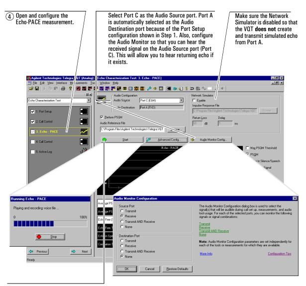
5 Start the Echo-PACE measurement. Test signals will be transmitted from the Audio Source port, and if or when echo returns, it will be analyzed and results will be displayed in the spreadsheet and the graph. Two examples of measurement results you might see are shown on the next two pages.
