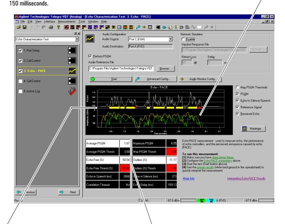
The VQT reports much more Echo in Speech and Echo in Silence when the returning echo's level is not attenuated much in relation to the test signal. Also notice that sharp increases in PSQM are more prevalent.
