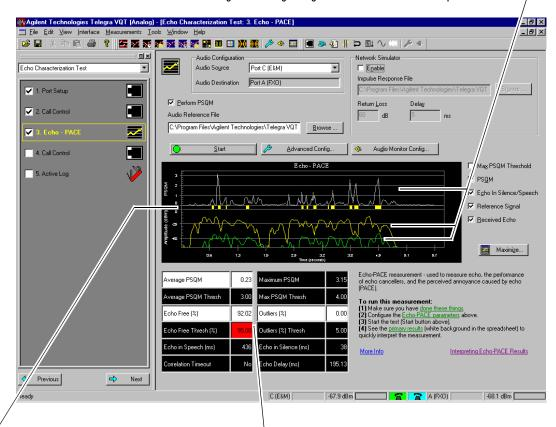
This band shows where the VQT reports periods of Echo in Speech and Echo in Silence. Echo in Speech and Echo in Silence results depend on user-defined thresholds that determine absolute signal levels and levels relative to the original test signal.
