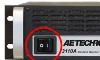
Figure 2.4 – 3110A on/off switch.
