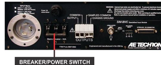
Figure 2.15 – System Component's Power/Breaker Switches and Gain Control (DSR 100-15 & 25 only)
