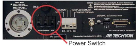
Figure 2.5 – Amplifier gain control and power switch.
