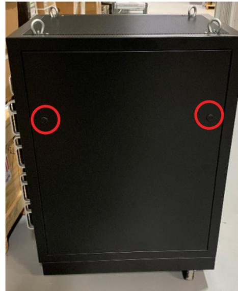
Figure 2.9 – Removing the right side panel
