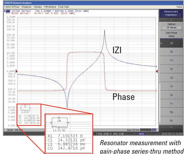
Resonator measurement with gain-phase series-thru method
