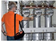
The measuring sensor extension (included in the scope of supply), which can be installed between the device and the measuring sensor, if necessary allows measurements on measuring points difficult to access.
