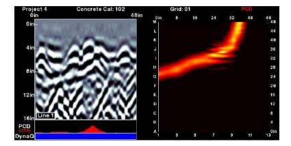
Power cables embedded in concrete pose an immediate risk when construction work needs to be done.
