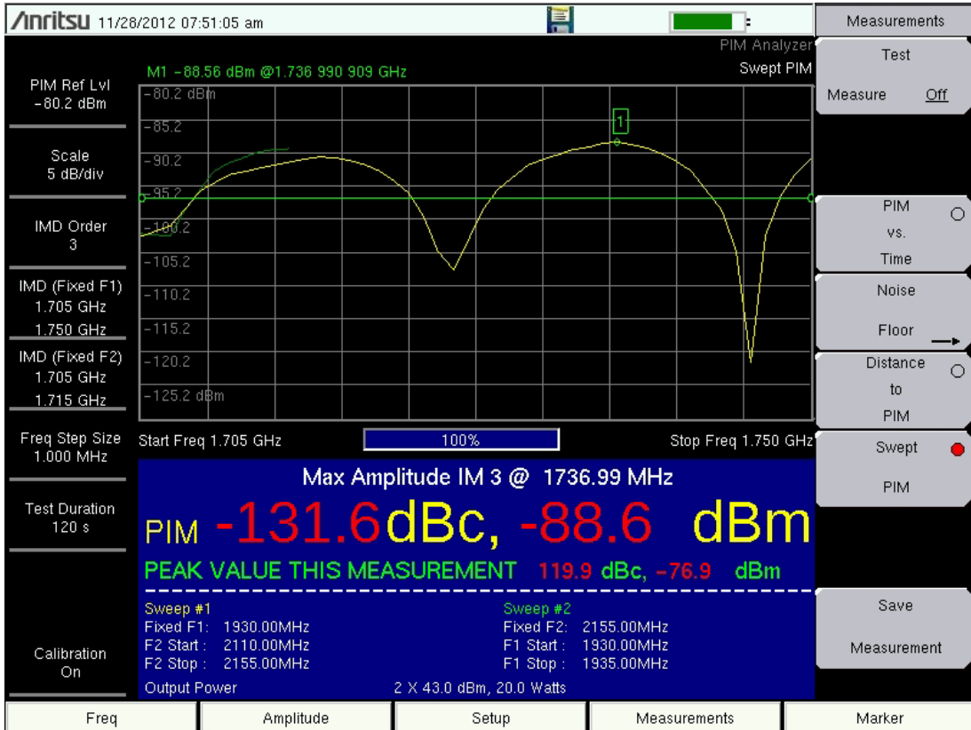
Figure 11-4. Swept PIM IM3 Measurement
