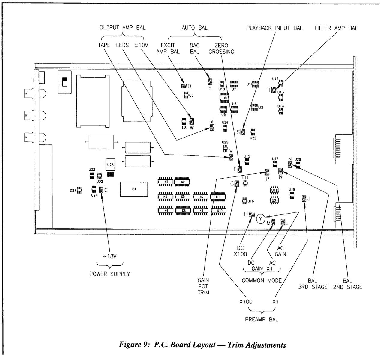
Figure 9: P.C. Board Layout — Trim Adjustments
