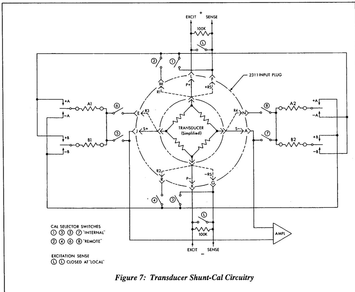
Excitation SENSE would be at LOCAL, unless the basic 6-wire system is in use, in which case it would be at REMOTE.
