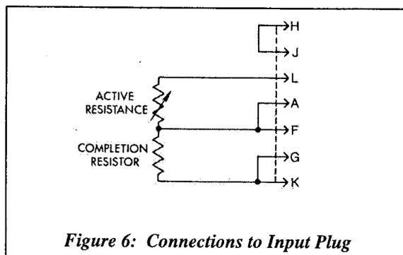
Figure 6: Connections to Input Plug
