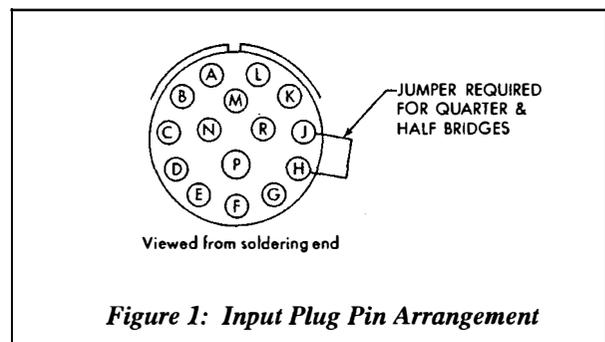
Figure 1: Input Plug Pin Arrangement
