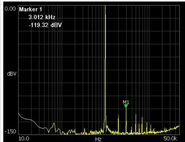
Figure 9. An FFT plot shows the residual distortion.
