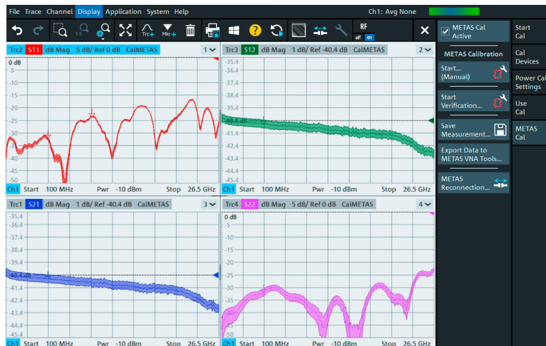
Real-time S-parameter measurements with uncertainty bands
