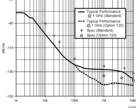
Residual FM 1 kHz RBW, 1 kHz VBW Option 1D5 Option 1DR Option 1DR and 1D5 System-related sidebands ≥30 kHz offset from CW signal
