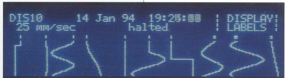
Fast, brilliant vacuum fluorescent monitor with 100 Hz refresh rate displays high frequency signals clearly in real time. The monitor also displays recorder menus for paperless setups.
