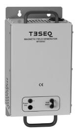
Its control is fully automatic, driven from NSG 3040 or NSG 3060 or WIN 3000. Once detected, the functions offered by MFO 6502 are available in the user interface or in the WIN 3000 software. As the voltage to A/m ration factor of the used loop antenna is available in the user interface or WIN 3000, the user will setup his tests directly in A/m, the software makes the calculation and drives the MFO 6502 to generate the right current through the loop antenna.
