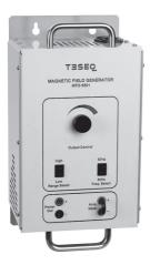
The MFO 6501 provides a convenient means of generating and adjusting the current to flow through one of the magnetic field loops, like INA 701 or INA 702 (see acces. sories). It is required for magnetic field testing for fields up to 40 A/m. It complies with the requirements of IEC 61000-4-8. It can be used as a stand alone instrument
