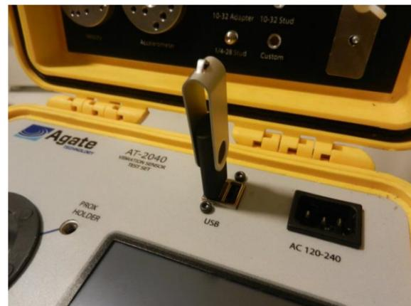
Figure 47. USB memory drive loaded in USB port
