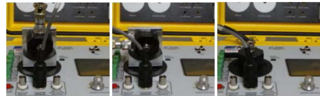
Figure 40. Sensor positioning and connection method
