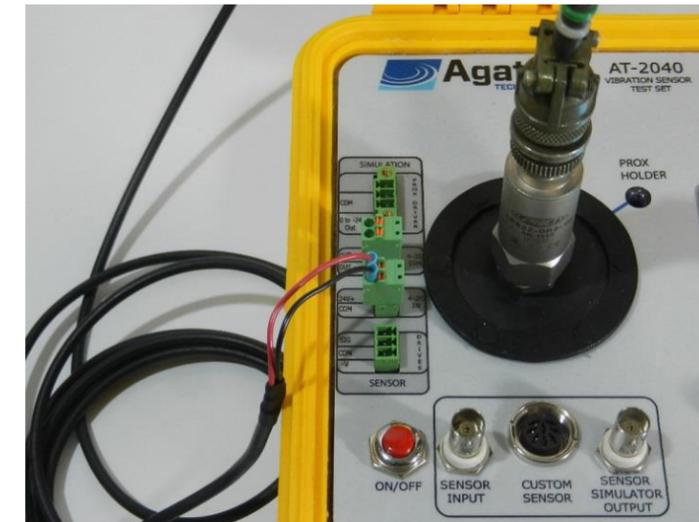
Figure 33. Sensor mounted to the AT2040
