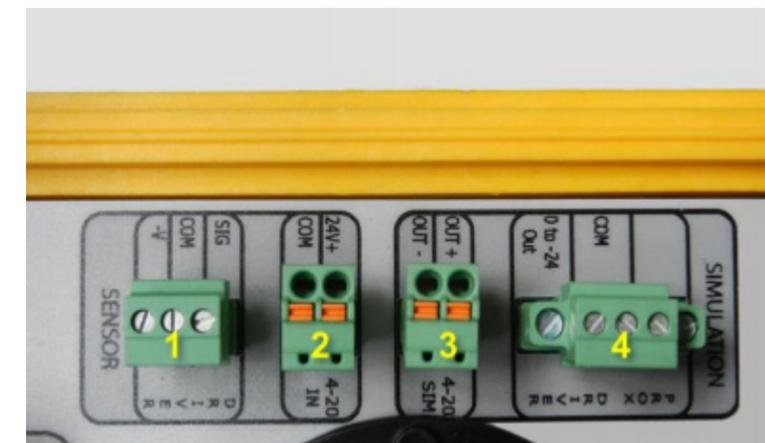
Figure 34. Connect the sensor to connector "2"
