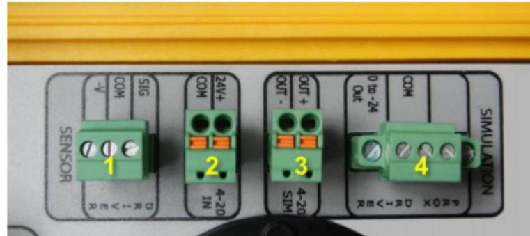
Figure 68. 4-20mA ("3") and proximity probe simulator connectors ("4")
