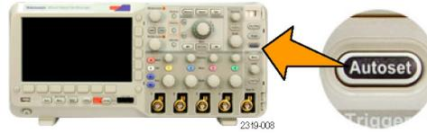
3. If desired, push **Undo Autoset** to undo the last Autoset.
