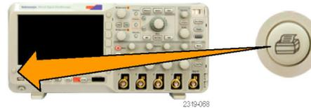
10. If printing fails, check that the USB cable is connected to the PictBridge port on the printer, and try again.
