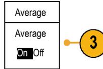
4. Turn multipurpose knob **a** to set the number of waveforms to average over.
