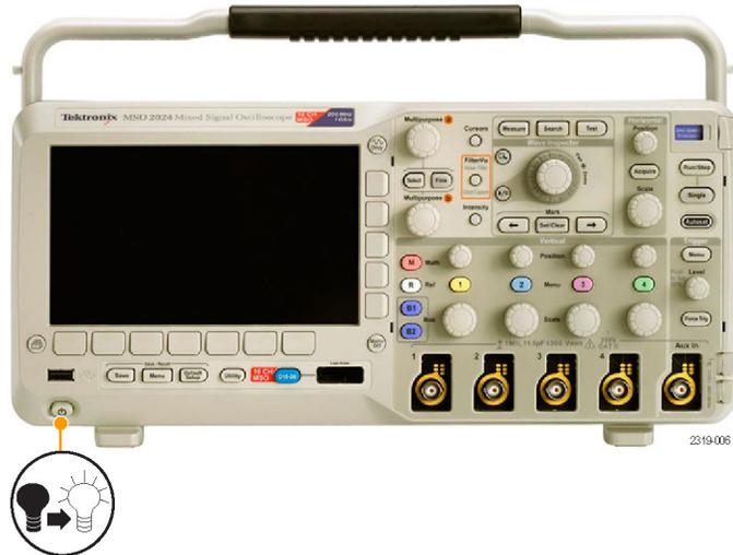
3. Connect the P2221 probe tip and reference lead to the **PROBE COMP** connectors on the oscilloscope.
