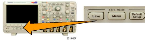
2. Push **Save Setup** or **Recall Setup** from the lower-bezel menu.
