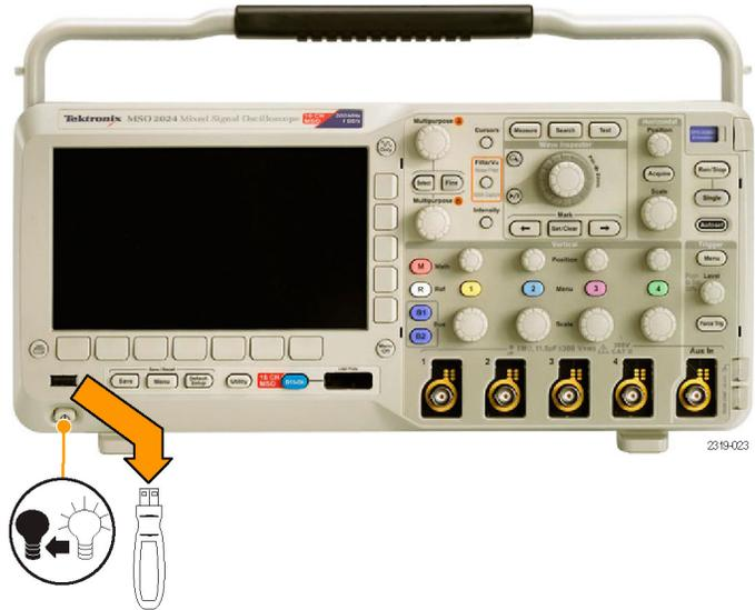
6. Power on the oscilloscope.
