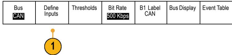
2. Turn multipurpose knob **a** to select the channel connected to the CAN bus source.
