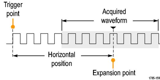
1. Adjust the position (delay) time by rotating the **Horizontal Position** knob.
