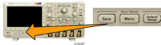
2. Push **Save Screen Image**, **Save Waveform**, or **Save Setup**.
