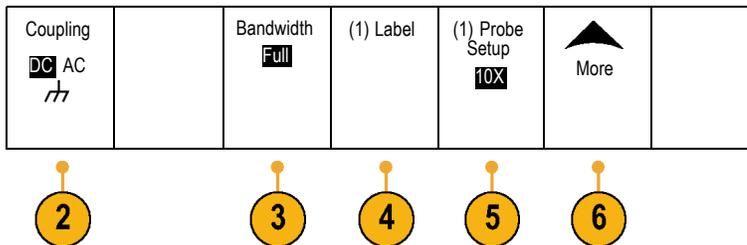
3. Push **Bandwidth**, and select the desired bandwidth from the resulting side-bezel menu.
