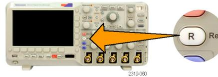
2. Push the **R1** or **R2** lower-bezel button to remove the reference waveform from the display.
