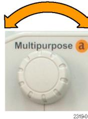
3. Turn multipurpose knob **b** to select the desired intensity for the graticule.
