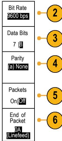
RS-232 decoding displays a stream of bytes. You can organize the stream into packets with an end-of-packet character
