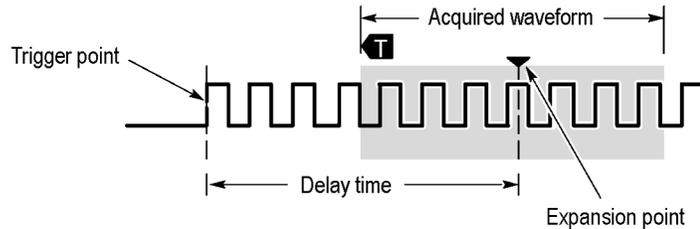
With **Delay** set to **On**, turn the **Horizontal Position** knob counterclockwise to increase the delay. The trigger point will move to the left and ultimately outside of the acquired waveform. Then you can adjust the **Horizontal Scale** knob to acquire more detail around the area of interest at the center of the screen.
