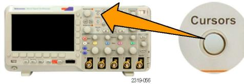
6. Turn multipurpose knobs **a** and **b** to move the pair of horizontal cursors.
