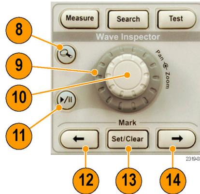
11. **Play-pause** button. Push to start or stop the automatic panning of a waveform. Control the speed and direction with the pan knob.
