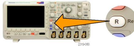
2. Use the resulting lower-bezel menu selections to display or select a reference waveform.
