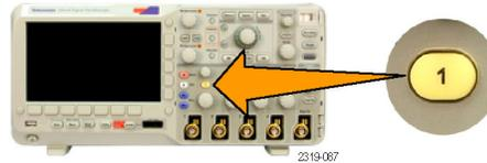
Connect the digital probe and select the input channel. (See page 112, *Setting Up Digital Channels (MSO2000 Series Only)*.)
