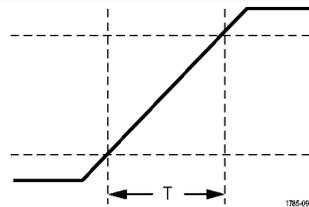
Trigger on rise and fall times. Trigger on pulse edges that traverse between two thresholds at faster or slower rates than the specified time. Specify pulse edges as positive or negative or either.
