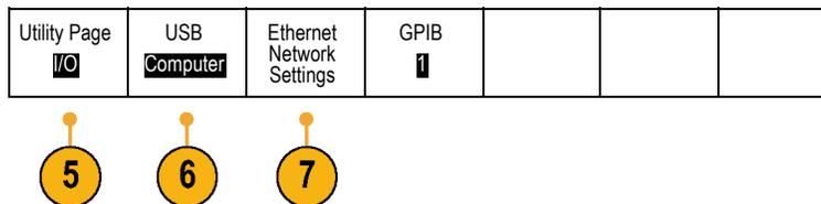
6. If a USB cable is connected between the oscilloscope and your computer, the oscilloscope automatically sets itself up for you.
