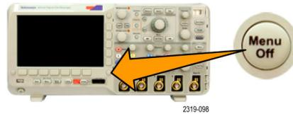
5. Certain menu choices require you to set a numeric value to complete the setup. Use the upper and lower multipurpose knobs and **a** and **b** to adjust values.
