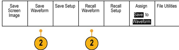
**NOTE.** The oscilloscope can save digital waveforms to .csv files, not reference memories. The oscilloscope cannot recall digital waveforms.
