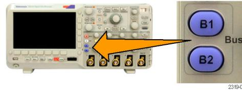
2. Push **Bus**. Turn multipurpose knob **a** to scroll through the list of bus types and select the desired bus: Parallel (MSO2000 series only), I<sup>2</sup>C, SPI, CAN, RS-232, or LIN.
