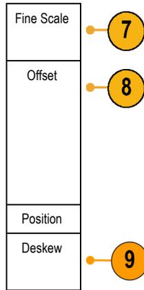
9. Select **Deskew** to set the time skew correction for the channel. Turn multipurpose knob **a** to adjust the time skew (deskew) correction for the probe attached to the selected channel. This shifts acquisition and display of the waveform left or right, relative to the trigger time. Use this to compensate for differences in cable lengths or probe types.
