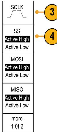
5. Use multipurpose knob **a** to set the number of bits to match the Word Size of the SPI bus.
