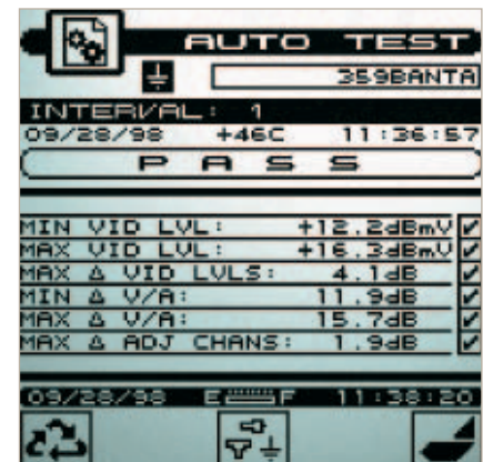
AUTO TEST results are time, date and temperature stamped and can easily be stored, viewed, printed (MS-1200D, MS-1300D, MS-1400) or uploaded to StealthWare software (MS-1300, MS-1400)
