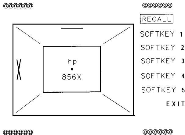
Figure 2-4. CRT Adjustment Pattern
