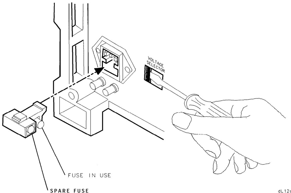
Figure 2-2. Voltage Selection Switch and Line Fuse Locations
