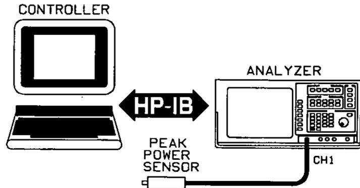
**Figure 6-1. Controller Setup**
