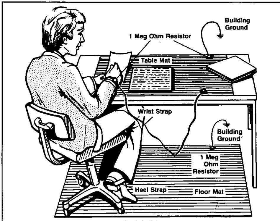
Figure 5-2. Static-Safe Workstation
