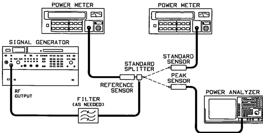
**Figure 6-3. Power Level Measurement Setup**
