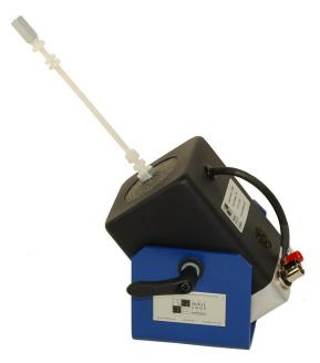
This electrodynamic exciter is a small, portable permanent magnet shaker with a new generation of ultra compact precision power amplifier integrated in its base. The revolutionary SmartShaker™ design eliminates the need for a separate, cumbersome power amplifier - just plug the excitation signal from a dynamic signal analyzer or function generator directly into the BNC on the base of the shaker. The unit is supplied with a DC power supply but can be run directly from any 12-21 VDC supply.
