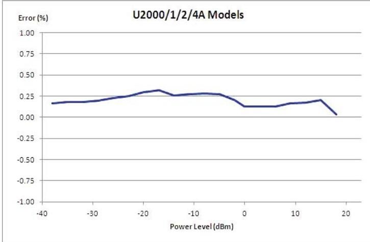
Typical power accuracy at 25 °C for U2000/1B sensors<sup>1, 2</sup>
