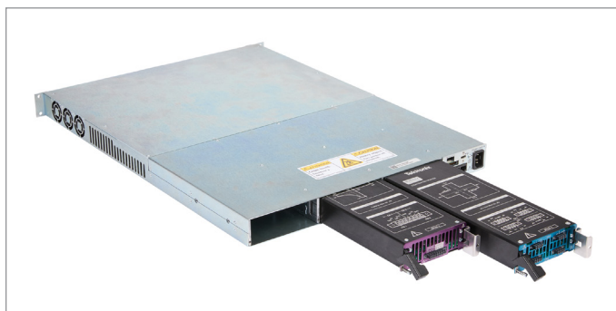
Figure 2: Rear View of MP5103 highlighting three module slots and simple module insertion and removal
