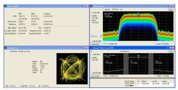
Time-correlated views in multiple domains provide a new level of insight into design problems not possible with conventional analyzers. Here, ACLR and modulation quality are performed simultaneously in a single acquisition, combined with the continuous monitoring of the DPX® spectrum display.
