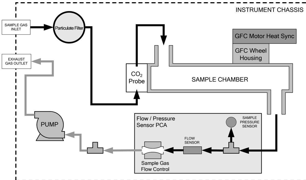
Figure 2-30. T300/T300M Internal Pneumatics with CO<sub>2</sub> Sensor Option
