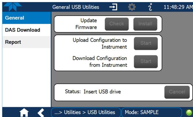
**Figure 2-61. Configuration Transfer**
