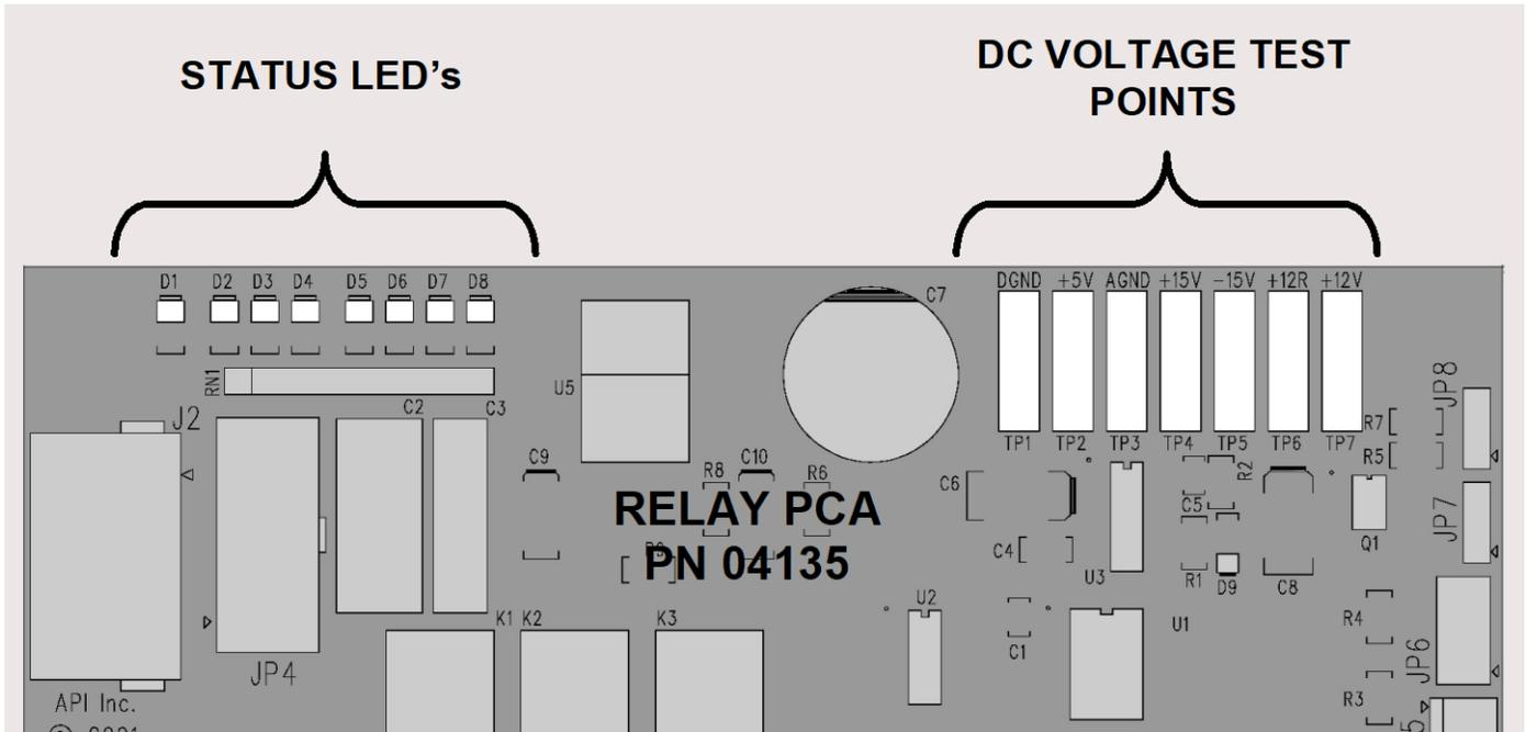
Figure 5-9. Relay Board Status LEDs
