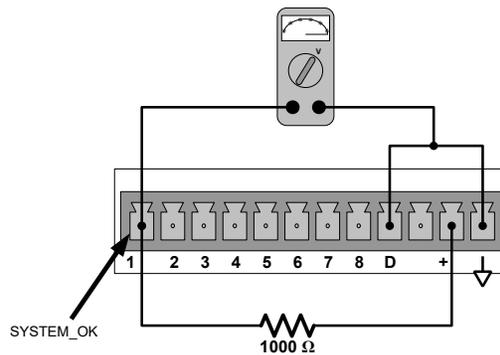
Figure 5-10. Typical Set Up of Status Output Test
