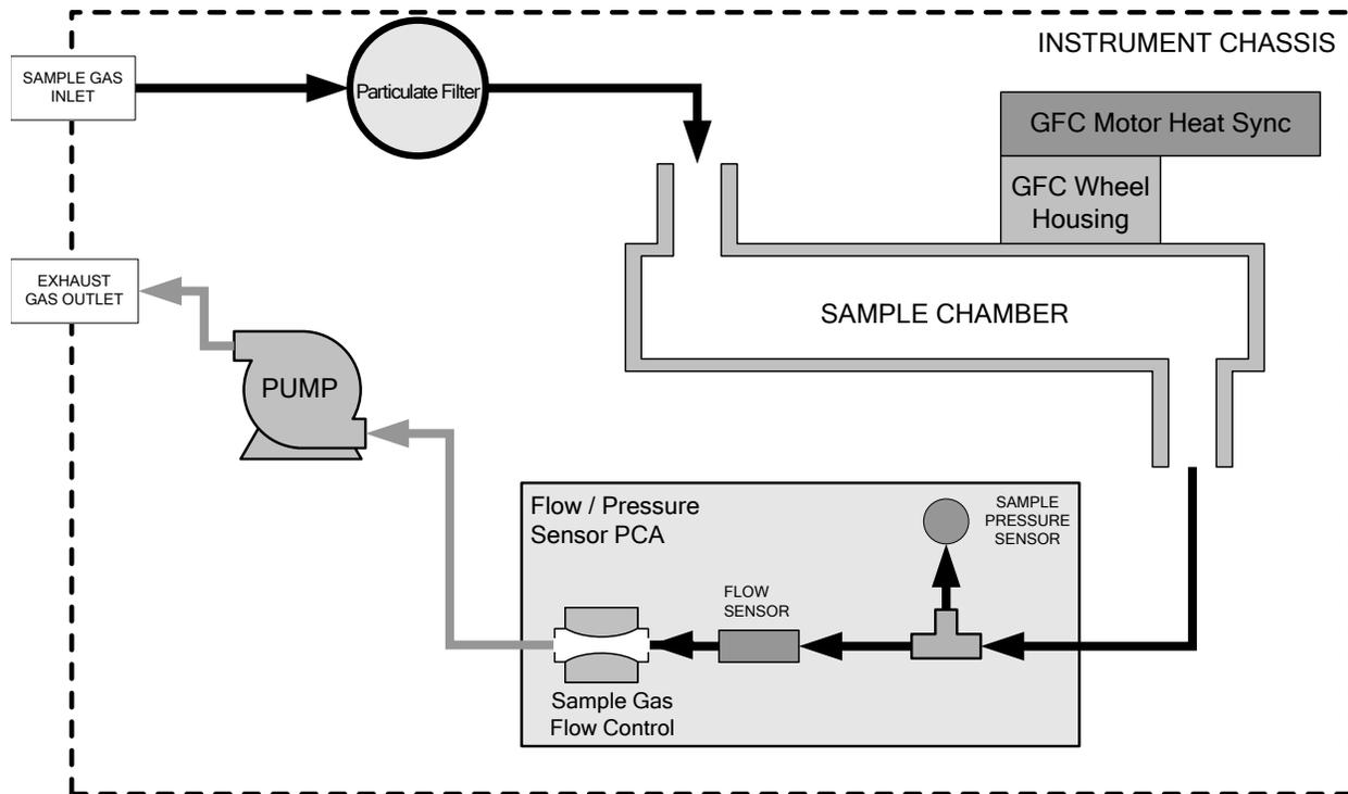
Figure 2-22. T300/T300M Internal Gas Flow (Basic Configuration)
