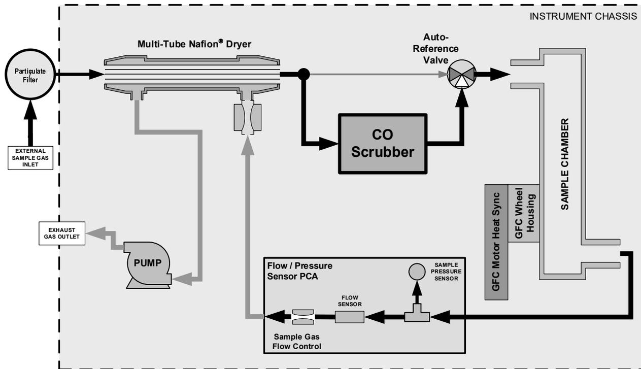
**Figure 6-7. T300U Gas Flow during Auto-Reference Measurements**
