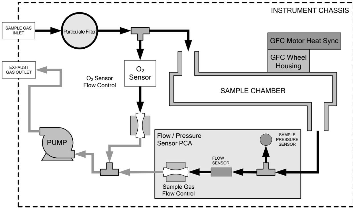
Figure 2-29. T300/T300M Internal Pneumatics with O<sub>2</sub> Sensor Option
