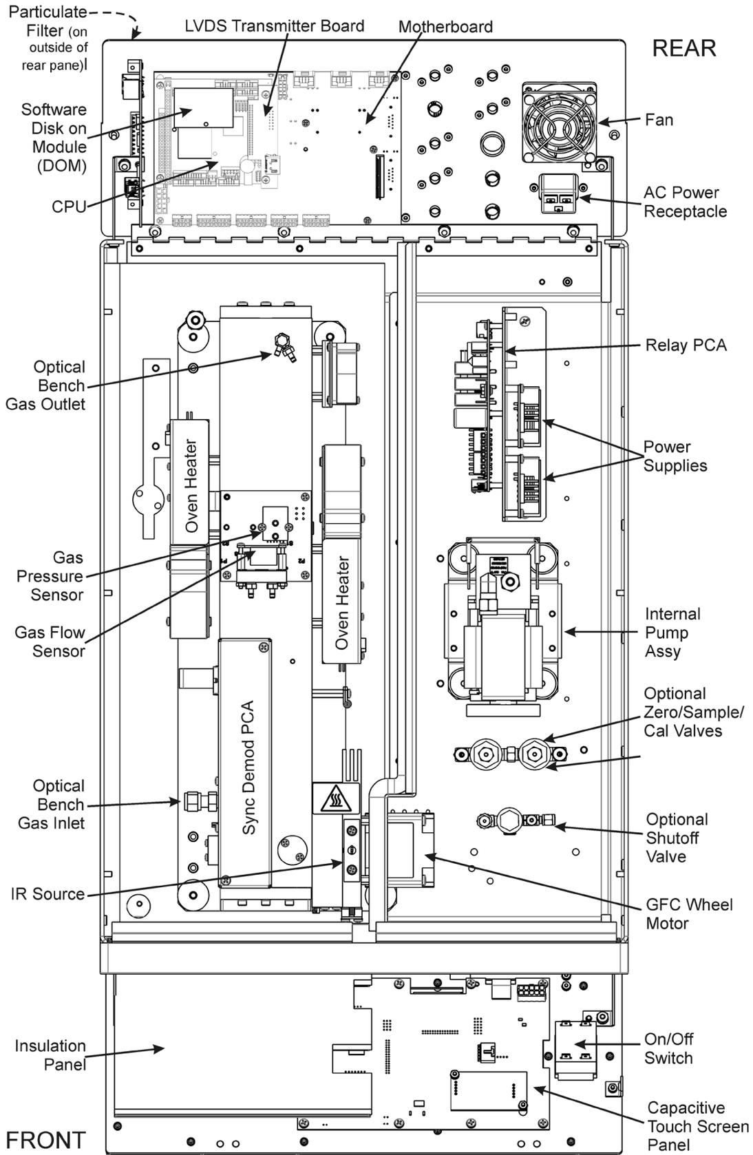
Figure 2-5. Internal Layout – T300U
