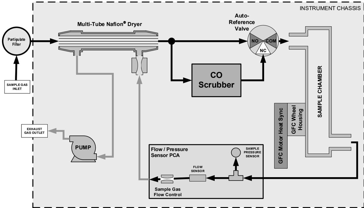
Figure 2-23. T300U Internal Gas Flow (Basic Configuration)
