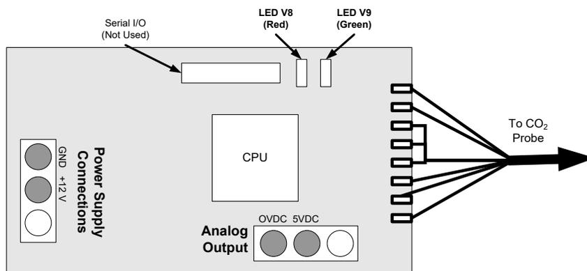
**Figure 5-11. Location of Diagnostic LEDs onCO<sub>2</sub> Sensor PCA**
