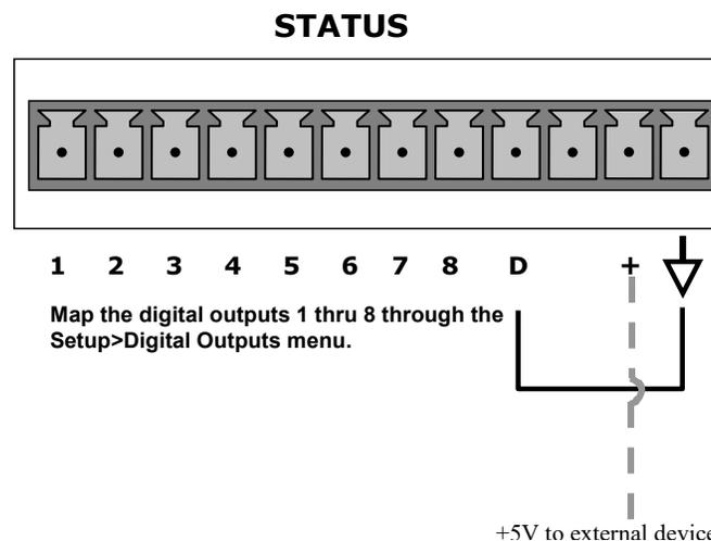
Figure 2-9. Status Output Connector for Digital Outputs
