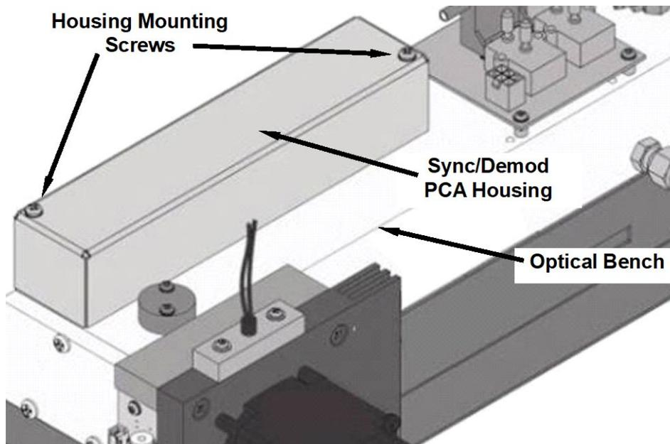
Figure 5-17. Location of Sync/Demod Housing Mounting Screws
