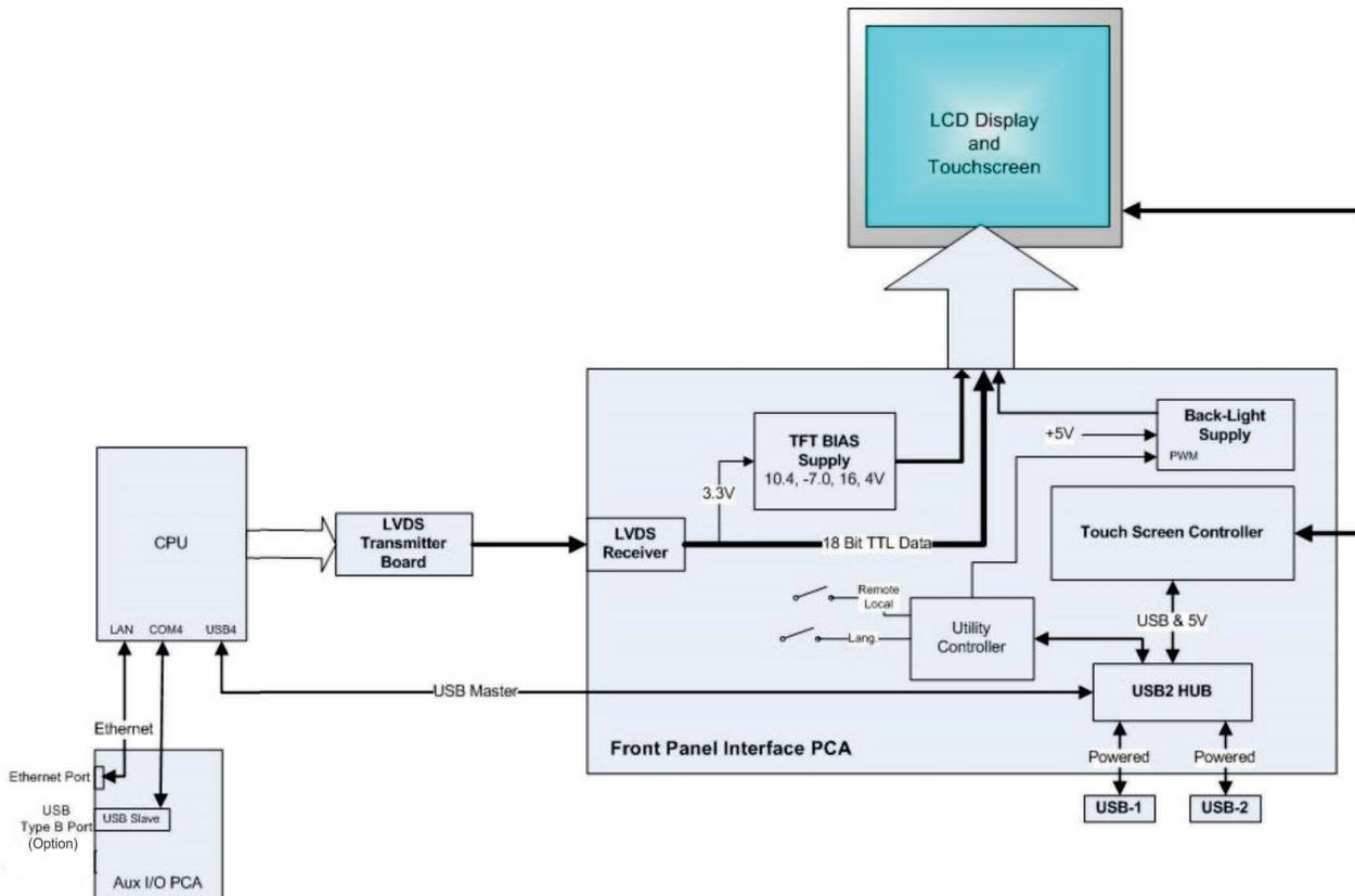
Figure 6-25. Front Panel and Display Interface Block Diagram
