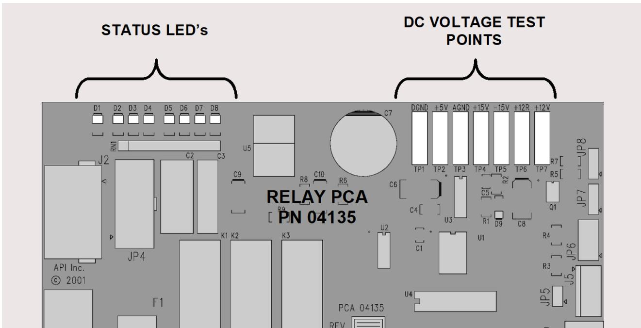
Figure 6-22. Location of relay board Status LEDs
