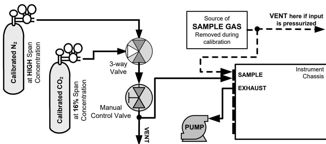
**Figure 4-5. CO<sub>2</sub> Sensor Calibration Set Up**
