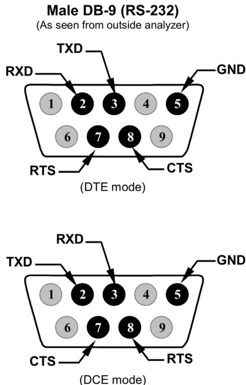
Figure 2-12. Rear Panel Connector Pin-Outs for RS-232 Mode
