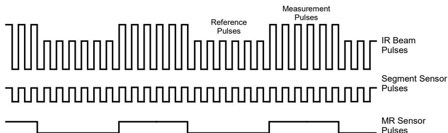
Figure 6-16. Segment Sensor and M/R Sensor Output
