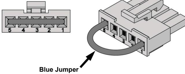
Figure 6-20. T300U Oven Heater Configuration Jumpers
