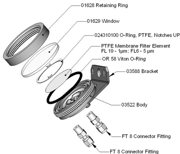
**Figure 5-6. Sample Particulate Filter Assembly**
