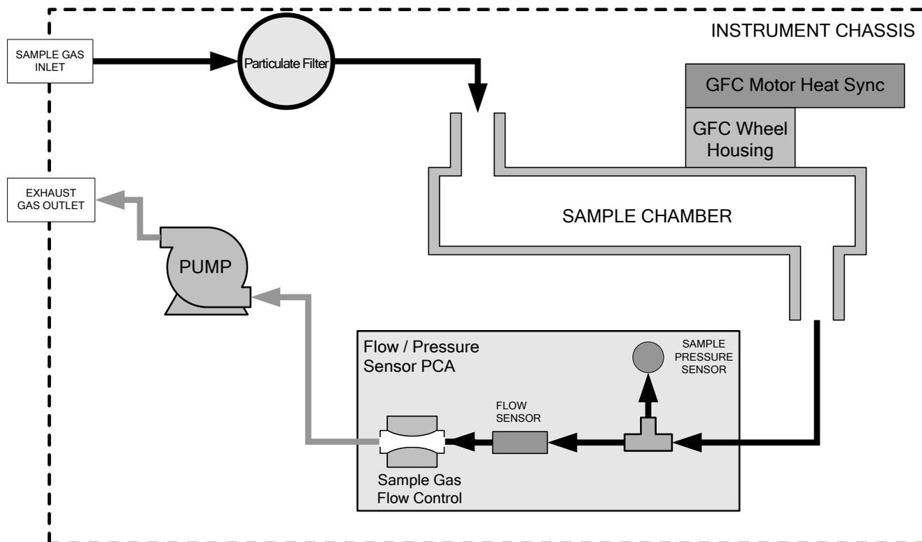
Figure 6-9. Internal Pneumatic Flow – Basic Configuration
