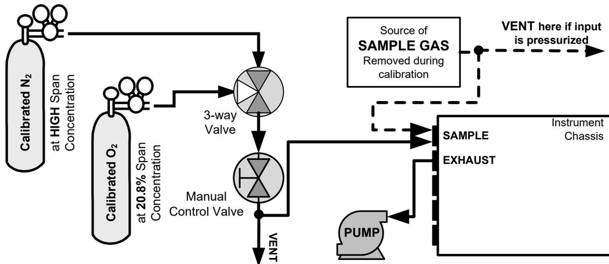
Figure 4-4. O<sub>2</sub> Sensor Calibration Set Up
