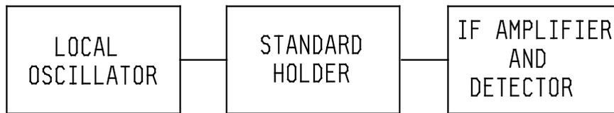
FIGURE 4121-1. Direct measurement method.
