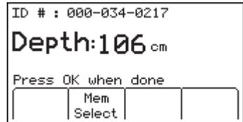
3. To save the depth reading, press *Mem Select* [SK].
