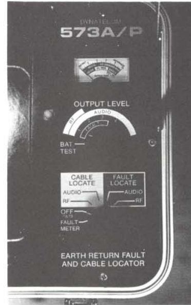
Fig. 9 — 573A/P Transmitter Unit Control Panel
