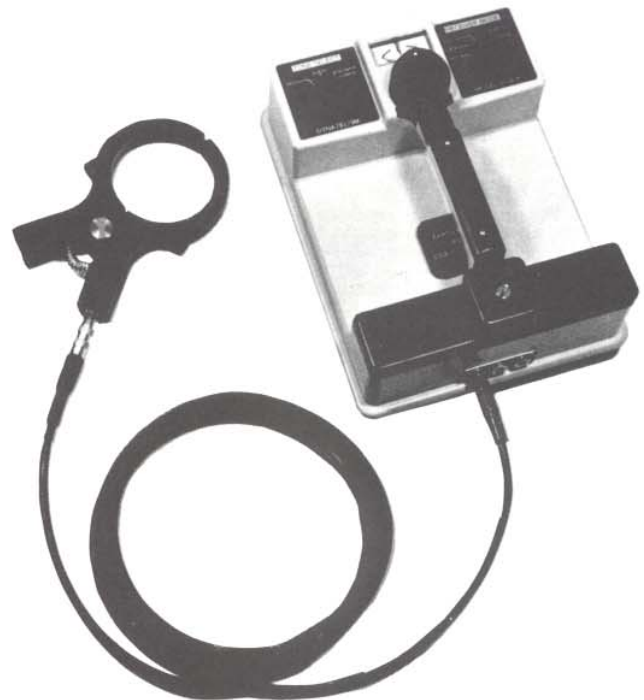
Fig. 26 — Receiver Setup for Cable Identification with a Dyna-Coupler®
