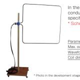
In the combination with LSS-6230, enable to conduct pulse magnetic field immunity test specified in IEC61000-4-9 Standard \* Scheduling to be released
