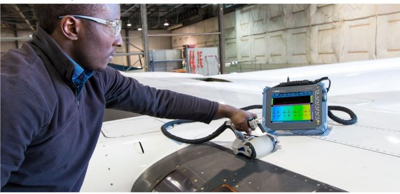
The RollerFORM™ phased array wheel probe from Evident is designed to address the inspection of composites and other smooth-surfaced materials. An affordable and easy-to-implement replacement for full 2D encoding systems, the RollerFORM scanner is a viable alternative to immersion techniques.
