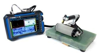
The RollerFORM™ scanner, combined with an OmniScan™ flaw detector, uses zero-degree ultrasonic beams for manufacturing and maintenance inspections. Common applications include delamination sizing and porosity quantification in composite core material, as well as wall-loss monitoring in metals.
