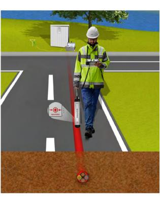
This means that the highly precise receiver is still able to deliver clear results in areas with lines that are routed closely together.
