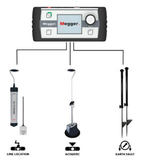
In addition to tracing and fault location, with audio frequency, it enables the user to acoustically pinpoint cable faults with great precision and accurately locate cable sheath faults using the voltage gradient method.
