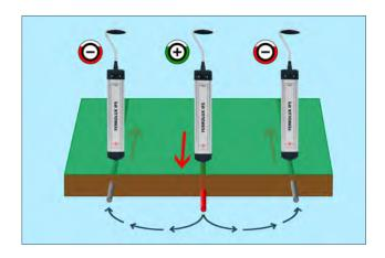
If there are several lines (cables, pipes) located next to each other, it is often difficult to determine which the correct one is. Sometimes the signal from the generator can flow through both lines, but the signal in the lines may be flowing in different directions. With the SignalSelect function, the generator applies a signal that contains direction information. When the device is positioned over the correct cable, a "+" symbol is displayed to facilitate precise identification.
