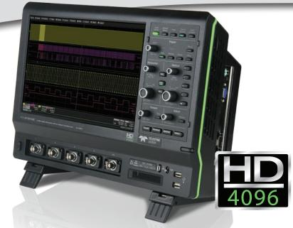
Combining Teledyne LeCroy's HD4096 high definition technology, with long memory, a compact form factor, 12.1" wide touch screen display, powerful debug tools, and mixed signal capability, the HDO4000 is the ideal oscilloscope for precise measurements and quick debug. Tools such as WaveScan Search and Find, LabNotebook Report Generator, and History Mode help identify and isolate problems for faster troubleshooting.
