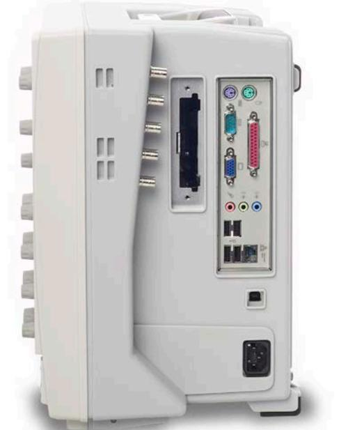
The Infiniium 9000 Series offers bandwidths up to 4 GHz. Each model, equipped with a large 15" XGA LCD display, comes in a whisper-quiet package that is just 9" (23 cm) deep and weighs only 26 pounds (11.8 kg).
