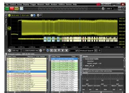
Trigger on and decode MIPI packets.
