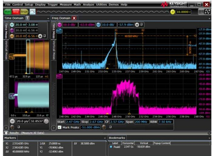
Mask tests, histograms and a wide variety of functions such as the gated FFTs in the above image provide deep signal analysis.
