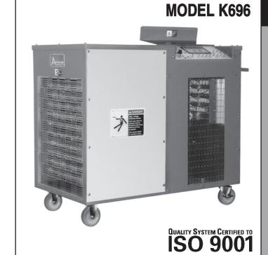
he Avtron Model K696 is a 250 KW portable load bank in a compact package weighing only 590 lbs. and only 44" high. One, two, or three K696 load banks providing 250, 500, or 750 KW can be transported to a job site in standard vehicles such as vans or pickup trucks. They do not have to be unloaded to enter underground parking garages.
