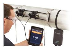
The Transport PT900 has the option for an energy measurement based on the temperature at a supply point, the temperature at a return point, and the flow of fluid through the system. This feature is specifically located in the PROGRAM OPTIONS section in the PROGRAM menu.
