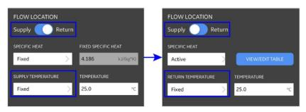
e. In the SPECIFIC HEAT section, open the drop-down list and select Fixed or Active as the type of supply for your system. If you choose Fixed, you will need to enter the desired value in the FIXED SPECIFIC HEAT section. If you choose Active, you will be able to enter up to six Temperature/SPECIFIC HEAT data points for your system in a table on clicking VIEW/EDIT TABLE as shown below.
