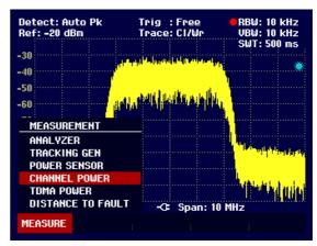
The R&S FSH3 displays the softkey menu for setting the channel power measurement. Two vertical lines in the measurement diagram indicate the channel bandwidth. The measured channel power is shown in large letters below the measurement diagram.
