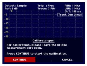
When OPEN calibration is over, the R&S FSH3 prompts the user to perform SHORT calibration.
