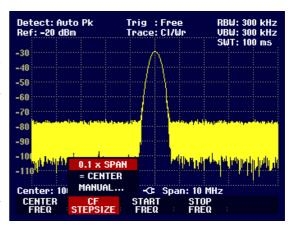
If you select "0.1 x SPAN" or "= CENTER", the R&S FSH3 makes the setting directly itself. If you select "MANUAL...", the value entry box opens and indicates the current stepsize.
