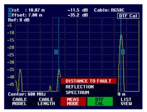
When SPECTRUM is selected, the R&S FSH3 turns off the tracking generator and displays the spectrum over the frequency range of the DTF measurement.
