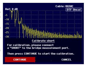
When SHORT calibration is over, the R&S FSH3 prompts the user to terminate the measurement plane with a 50  $\Omega$  Load.
