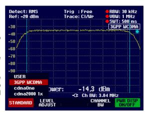
If USER is selected, the R&S FSH3 sets the last channel power measurement setting used in the USER mode. The R&S FSH3 automatically makes changes to the setting so that it is again available when the USER standard is called again.
