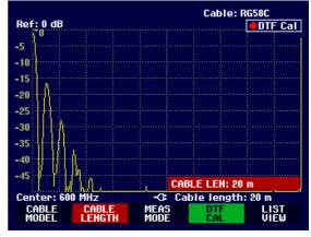
N.B.: The cable length should be entered before the test setup is calibrated. If it is entered afterwards, the measurement accuracy is reduced.
