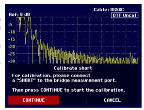
While SHORT calibration is in progress, the R&S FSH3 outputs the message "Calibrating SHORT, please wait...".
