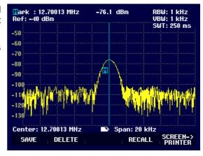
➤ The SCREEN->PRINTER softkey starts the screenshot printout on a printer.
