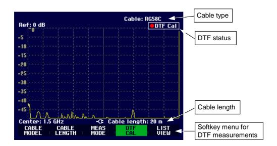
To perform distance-to-fault cable measurements, the R&S FSH3 needs to "know" the type of cable and its approximate length.
