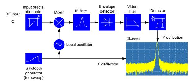
The precision attenuator at the input of the Spectrum Analyzer adjusts the level of the measurement signal to the level range that the mixer can handle without overdriving it. The precision attenuator at the input of the R&S FSH3 is adjustable in 10 dB steps from 0 dB to 30 dB and is directly coupled to the reference level setting.
