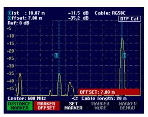
As is the case with spectrum analysis, the R&S FSH3 provides functions to automatically position the marker or the marker offset on the trace. These can all be accessed by pressing the SET MARKER softkey.
