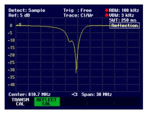
The transmission calibration remains valid until the R&S FSH3's Center Frequency or span are changed. If calibration becomes invalid, the R&S FSH3 displays Track Gen Uncal in the top right-hand corner of the screen.
