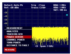
The R&S FSH3 opens the screen for power measurements. If a power sensor has not been connected, no measured value is displayed. If a power sensor has been connected, the R&S FSH3 sets up a connection via its interface and after a few seconds displays the measured power.
