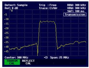
The transmission calibration remains valid until the Center Frequency or the span is changed on the R&S FSH3. Track Gen Uncal is displayed in the top right-hand corner of the screen when calibration is no longer valid.
