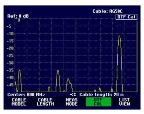
The R&S FSH3 can also list any cable faults. It displays the return loss and distance from the measurement plane of all reflections that exceed a settable threshold.
