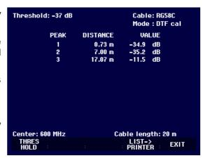
The distance to the cable faults or the distance between any two faults can also be read off with the marker.
