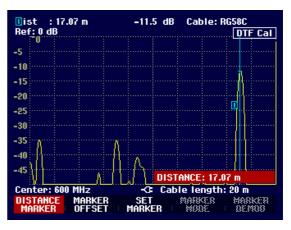
The reference plane to which the distance of a reflection is referred can be redefined using the marker offset.
