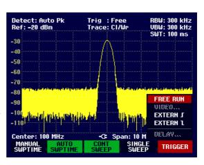
If the VIDEO... trigger setting has been selected, the trigger level and any trigger delay (DELAY...) must be entered. The trigger level is expressed as a percentage (%) of the reference level. 100% means that the trigger level equals the reference level, 50 % that the trigger level is in the middle of the y axis on the measurement diagram (default setting). The position of the video trigger on the level axis is shown by a ">".
