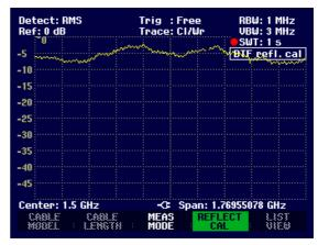
Checking the spectrum in the frequency range for detecting external interferers:
