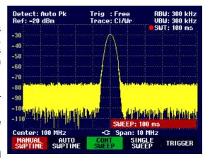
Whenever a change is made, the sweep time is immediately set to its new value. The value entry box is closed by pressing the ENTER key. The sweep time that has been set is displayed in the top right-hand corner of the screen in the SWT readout box.
