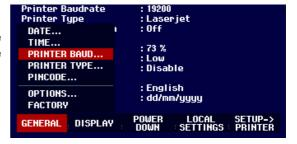
The selection box for the baud rates available (1200 baud to 115200 baud) opens.
