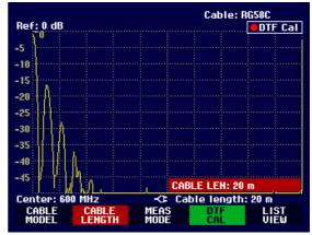
N.B.: The cable length should always be entered before the test setup is calibrated. If it is entered afterwards, the measurement accuracy is reduced.
