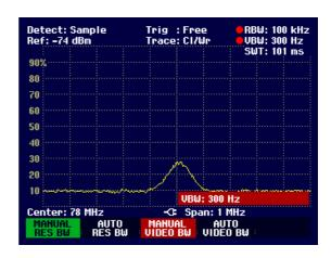
Limiting the Video BandWidth smoothes the trace considerably. This makes it much easier to determine the level of the measured signal.
