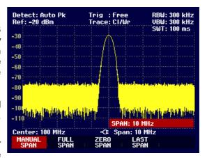
Use the FULL SPAN softkey to select the full Span from 0 Hz to 3 GHz with a single keystroke.
