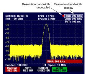
The box for entering the Resolution BandWidth can be closed by pressing the CANCEL key.
