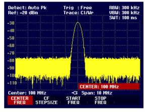
The smallest step for adjusting the Center Frequency with the Rotary knob is a pixel, in other words, as the trace comprises about 300 pixels, each step is equal to about 1/300 of the Span. When you use the Cursor keys, a frequency step is equal to 10 % of the Span (= 1 grid division). If you want to use a different step size, you can define it with the CF STEPSIZE function (CF= Center Frequency).
