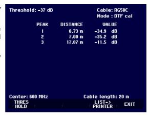
The distance to the cable faults or the distance between any two faults can also be read out with the marker.
