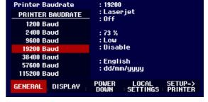
Note: If the serial/parallel converter (R&S FSH-Z22) is used to control a printer with a parallel interface, set the RS232 interface to 38400 baud.
