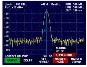
The R&S FSH3 now displays the counted marker frequency with a resolution of 1 Hz. To indicate that the FREQ COUNT function is on, Mark in the top left corner of the screen changes to **Count:**
