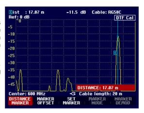
Checking the return loss of the cable under test:
