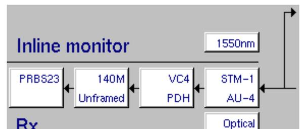
Terminated testing requires that live traffic be removed from the circuit before testing can begin. This frees the circuit for advanced testing techniques such as injecting test patterns or manipulating bit values. By simultaneously generating and analysing the received data for errors, the ANT 5 can analyse the performance of the circuit in both directions.
