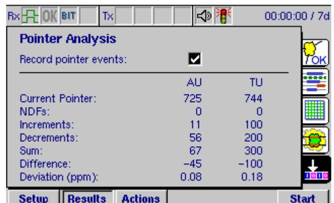
ANT-5 displays the current pointer value together with counts of the numbers of **Increments** (+PJE), **Decrements** (-PJE) and **New Data Flags** (NDFs). The **Sum** is the number of increments and decrements, the **Difference** is the number of increments less the number of decrements. The **Deviation** (in ppm) is the number of times the pointer has moved in relation to the number of bits received. By checking the
