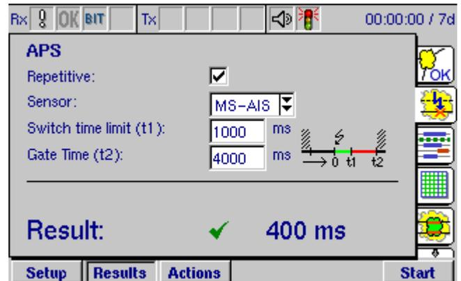
Detection can be achieved by monitoring the reduction in Quality of Service (QoS) or monitoring the resultant alarms. Depending on the signalling structure the following **sensors** can be selected, TSE, MS-AIS, AU-AIS, TU-AIS and Service Disruption. When selecting Service Disruption, the sensor activates upon detecting any of the following events: TSE, AIS, LOS or LOF.
