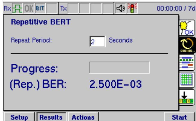
A **Repeat Period** of 1 second is adequate for measuring high error rates, but this period can be adjusted to a maximum of 99 seconds to test for lower rates.
