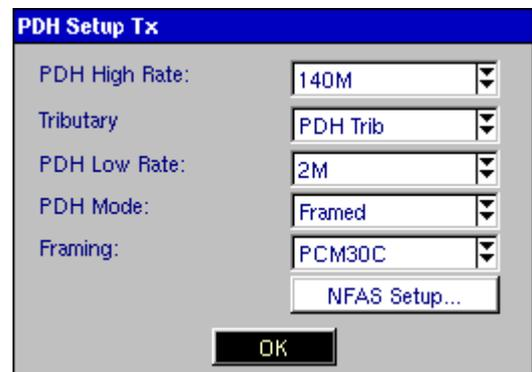
The generation feature allows the insertion of alarms and errors at all levels in the chain (including E2).
