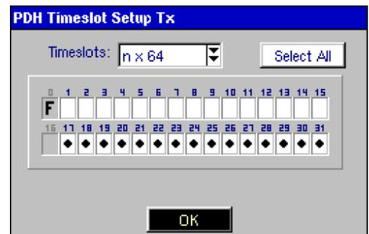
**Note:** The ANT-5 will only be able to transmit and receive nx64 when E1 framing is part of the hierarchy. Channel 0 is used for FAS/NFAS and will always be greyed out; channel 16 (used for signalling purposes) will be greyed out if either PCM30 or PCM30C are selected as part of the framing structure.
