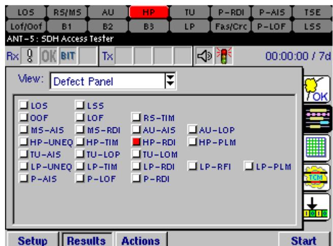
**Note:** Defect panel LED's turn yellow during a test to show historic alarms, that is, defects that have been raised during a test but are not currently active. To reset the LEDs press **Alt** and **Menu** and select **System >LEDs >Reset LEDs**.
