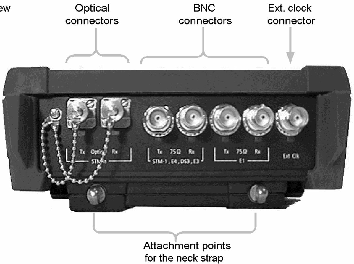
The ANT-5 has the following external connectors on the left side:
