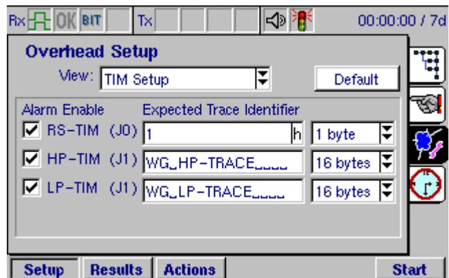
If the RS-TIM is set to 1 byte, its contents are entered in the form of two hexadecimal digits. During this entry, the function keys are temporarily assigned the alphabetical values 'A' to 'F'. The two hexadecimal digits can be entered by using the keyboard for the decimal numbers and the function keys for the alpha characters.
