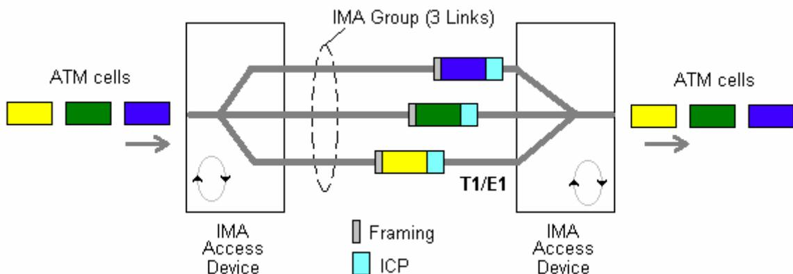
IMA defines two new types of OAM cells, the filler cells and the ICP cells. The filler cell (53 bytes) is used for rate decoupling at the IMA sublayer. The ICP cell (53 bytes) contains information about the IMA link and is available on each link belonging to the group.
