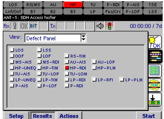
**Note 1:** PLM, UNEQ and TIM alarms are associated with G.832 framing in PDH E3 or E4 mode. If these alarms are generated the **HP** soft led situated at the top of the screen will light up.
