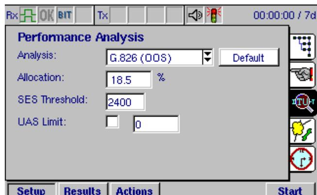
**SES Threshold** allows setting of the threshold for Severely Errored Seconds, which in G.826 is said to be 30% of the number of blocks in one second.
