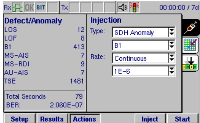
The number of anomalies to be injected is selected from the **Rate** list box and can be set to **Single** or **Continuous**. The **Continuous** rates available are **1E-2**, **1E-3**, **1E-4**, **1E-5**, **1E-6**, **1E-7**, **1E-8**, **1E-9** or **1E-10**, the available rates depending upon which anomaly is selected.
