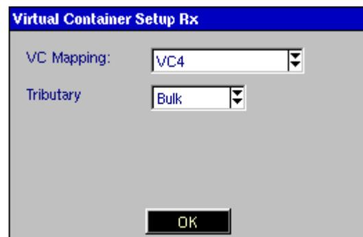
If testing within a PDH hierarchy is required, the **PDH** tributary should be selected. The test pattern will then be injected into the selected SDH virtual container with the selected PDH parameters.
