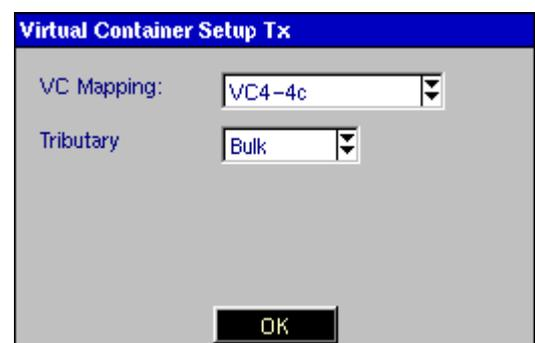
A test pattern can be injected throughout the contiguous concatenated payload of the Virtual Container in either transmit or receive mode as required.
