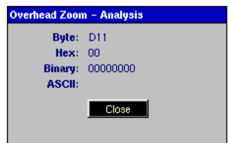
Where an overhead byte is used for a special purpose, such as carrying status messages (S1) or labels (C2), these values will also be displayed and alternative values may be selected from a list.
