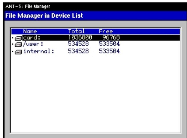
**Note 1:** The **user:** device is the internal RAM storage. In normal circumstances the ANT-5 operating system copies the data stored in this area into non-volatile memory during its power-down sequence. Data may be lost from this device in exceptional circumstances when the power-down is not controlled by the operating system, for example if the ANT-5 is switched off by holding the **Off** key down for more than 6 seconds.
