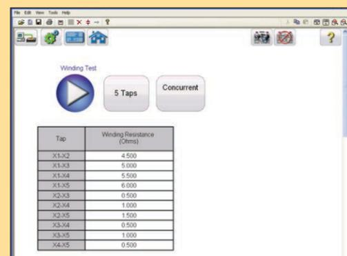
Winding Resistance test screen
