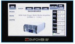
The **Dashboard** is your quick at-a-glance system status showing output power, reflected power, input power, internal temperature, transistor drain current, and transistor drain voltage.
