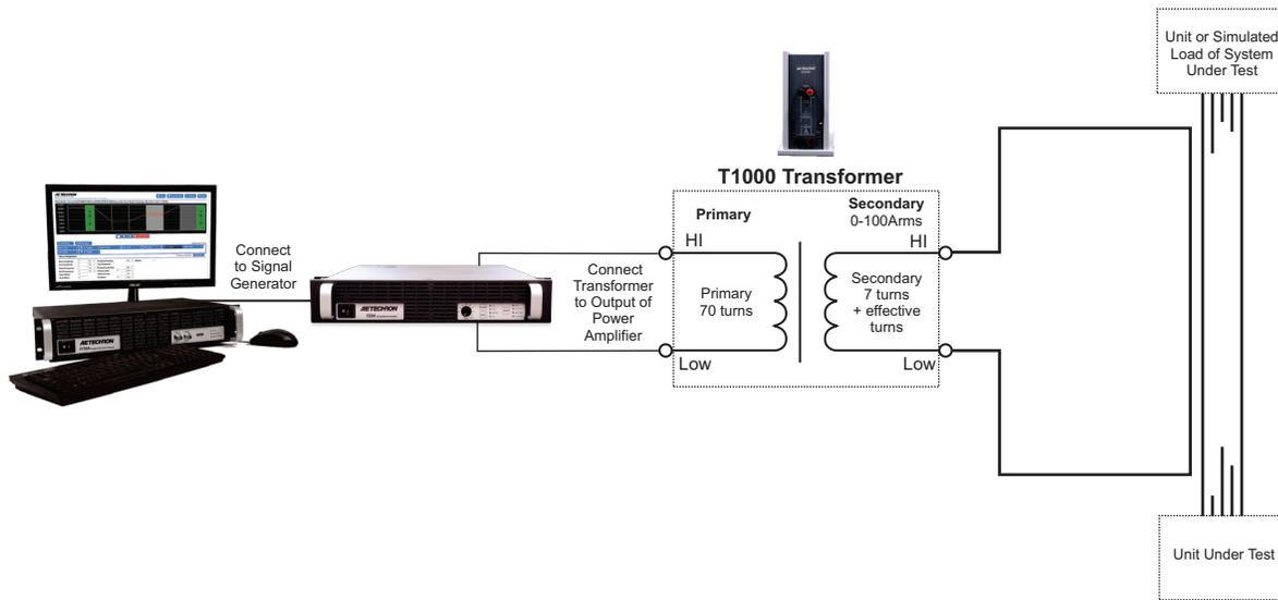
Figure 2 – Sample Application: DO 160 Section 19 Test Load Wiring
