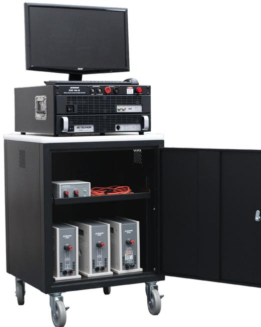
The **CIS-25 Test Kit** combines into a single, complete package the items needed to accurately test to important Aviation standards like DO-160 sections 18 and 19.
