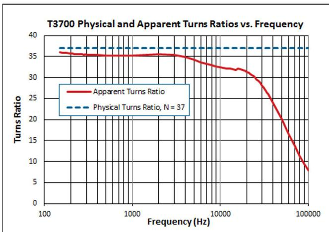
Figure 3 – Physical and Apparent Turns Ratios vs. Frequency
