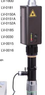
Installing the LV-0181 (Built-in positioning camera), the LV-0185 (Illumination unit) and an objective lens to the LV-1800 enables micro spotting of laser beams and image observation by epi-illumination. It makes laser positioning to microstructures and detection of multipoint parts possible.
