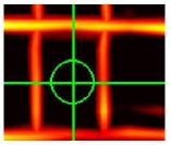
Decide exactly where to drill in the grid with the drill locator with variable drill bit diameters
