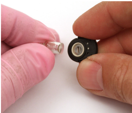
Figure 31: Reinstalling the Electrode Lamp
