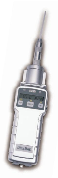
UltraRAE is a quick, spot-check monitor, typically used by occupational health, safety and environmental personnel. The combination filter tube and PID removes the disadvantages associated with colorimetric tubes and gas chromatographs. Applications include tank entry pre-screening during refinery and plant maintenance, hazardous material response, marine spill response and refinery down-stream monitoring.
