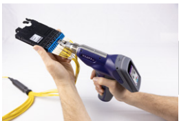
Inspect Duplex Connectors
