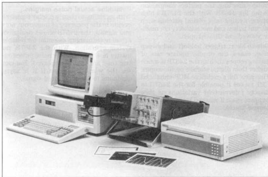
The 2467B and Tek DCS01 Digitizing Camera System combine to give you 400 MHz single-shot capability along with up to 10 ps/point digitizing.
