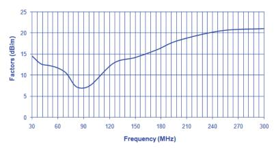
Field strength (dBV/m) = Output measured (dBV) + Antenna Factor (dB/m)
