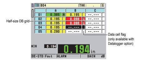
Figure 9-7 Example of the half-size DB grid
