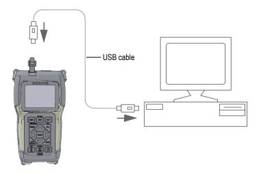
Figure 11-1 Connecting the 45MG to a computer
