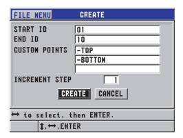
Figure 6-20 Configuring ID range for a sequential with custom points data file type
