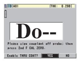
Figure 6-6 Opening the THRU-COAT setup dialog box
