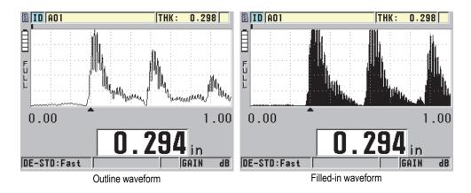
Figure 6-10 Examples of waveform trace modes
