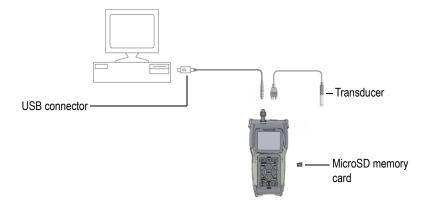
Figure 1-2 The 45MG connections
