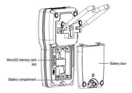
Figure 1-4 The MicroSD connector behind the battery door
