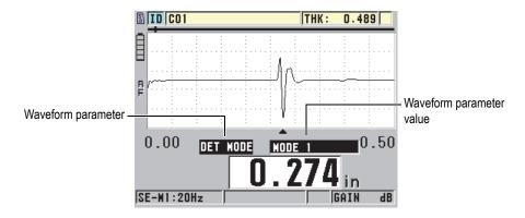
Figure 10-2 Adjusting the waveform parameters
