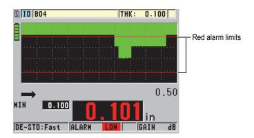
Figure 7-5 Example of a B-scan alarm mode
