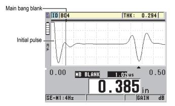
Figure 10-9 Main bang blank position for mode 1
