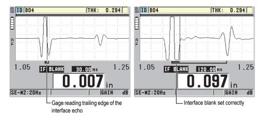
Figure 10-14 Examples of the interface blank in mode 2
