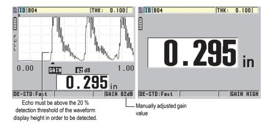
Figure 9-1 Manually adjusting the gain
