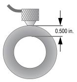
Figure 5-11 Coupling a dual element transducer
