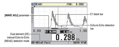
Figure 6-4 Measuring with the manual Echo-to-Echo detection mode
