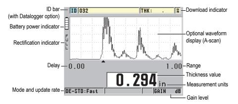
Figure 3-2 The measurement screen – Waveform option enabled
