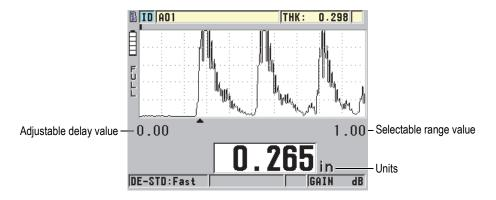
Figure 6-11 The range of the waveform display
