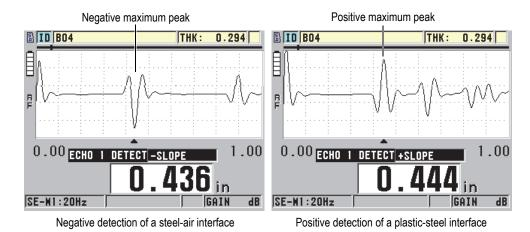
Figure 10-13 Negative and positive echo detection examples
