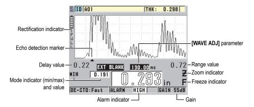
Figure 3-5 Other elements – Waveform option enabled
