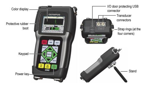
Figure 1-1 The 45MG hardware components – Front, top, and side views
