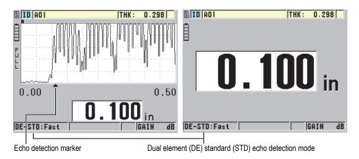
Figure 6-2 Measuring with the standard echo detection mode
