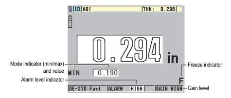
Figure 3-4 Other elements – No Waveform option enabled
