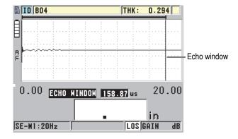
Figure 10-11 Echo window setting for mode 1
