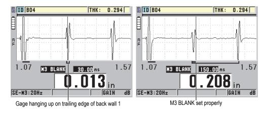
Figure 10-16 Examples of M3 Blank adjustment
