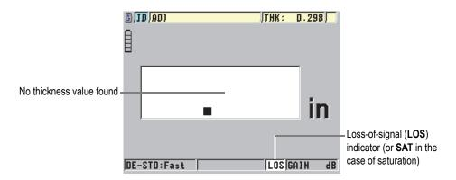
Figure 3-6 The loss-of-signal (LOS) indicator
