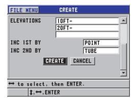
Figure 6-25 Configuring the ID range for a boiler data file type
