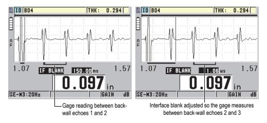
Figure 10-15 Examples of the interface blank in mode 3
