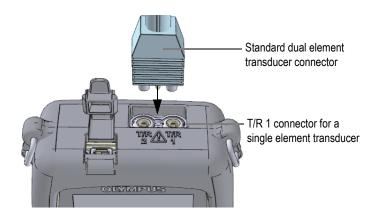
Figure 5-1 Plugging in the transducer
