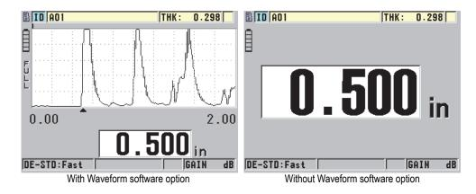
Figure 5-12 Reading the measured thickness
