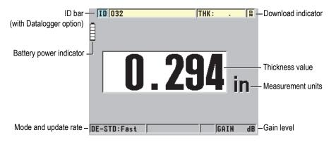
Figure 3-1 The measurement screen - No waveform enabled
