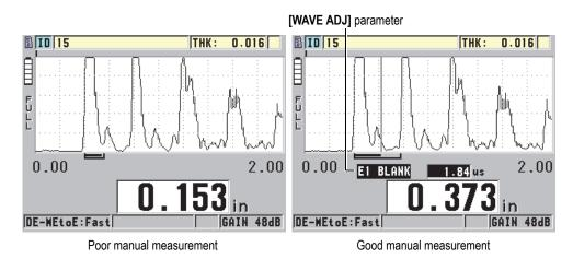
Figure 6-5 Comparing manual measurements
