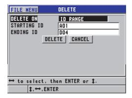
Figure 6-32 Deleting the data of an ID range in the active file
