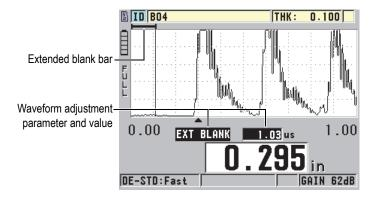
Figure 9-2 Adjusting the extended blank length
