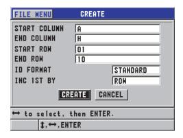
Figure 6-24 Configuring the ID range for a 2-D grid data file type
