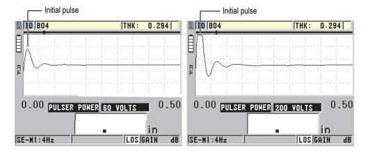
Figure 10-7 Comparing pulser powers set to 60 V and 200 V
