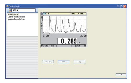
Figure 11-5 The Device Tools dialog box with a screen capture
