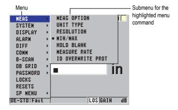
Figure 3-7 Menu and submenu example
