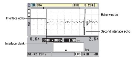
Figure 10-12 Echo window setting for mode 2 and mode 3
