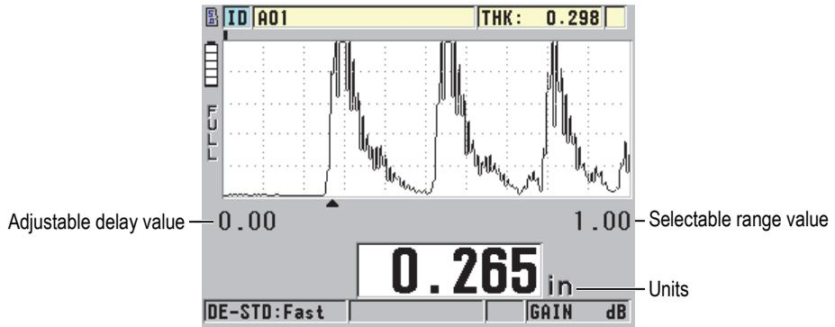
Figure 6-11 The range of the waveform display
