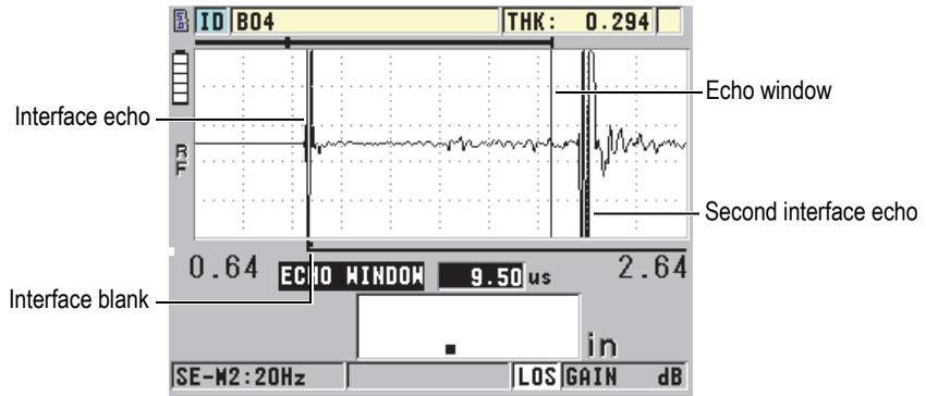
Figure 10-12 Echo window setting for mode 2 and mode 3
