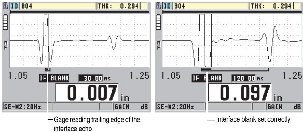
**Figure 10-14 Examples of the interface blank in mode 2**
