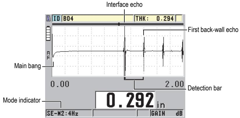
**Figure 10-4 Mode 2 detection example**
