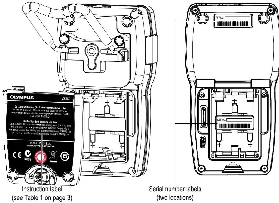
Figure i-2 Labels attached to the back of the instrument
