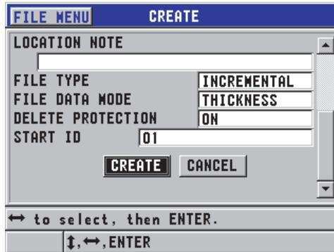
**Figure 6-18 The CREATE screen for the incremental data file type****6.7.2.3 About the Sequential Data File Type**
