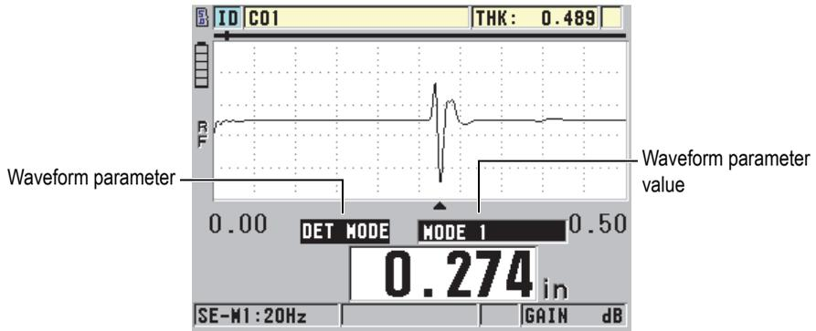
Figure 10-2 Adjusting the waveform parameters
