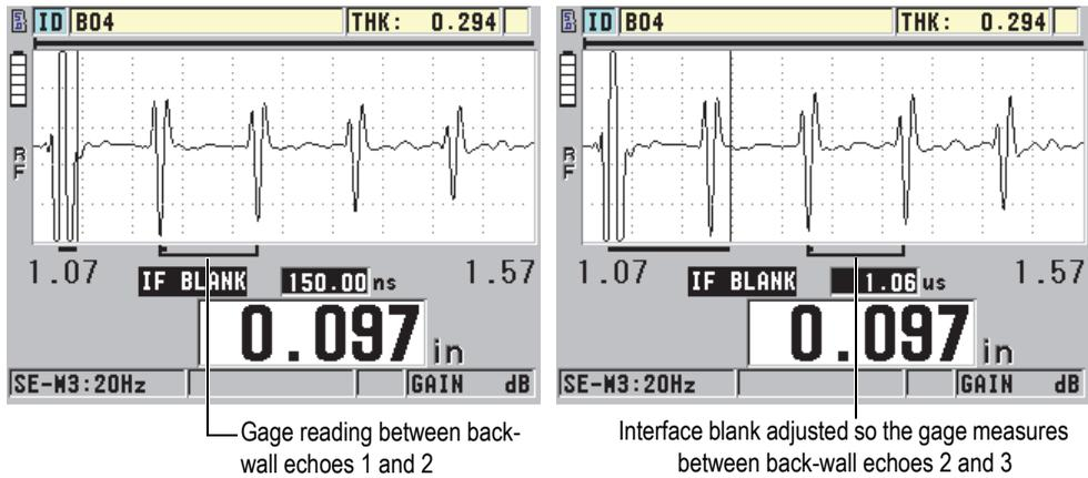
Figure 10-15 Examples of the interface blank in mode 3
