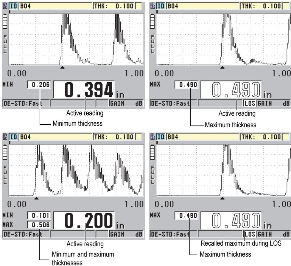
**Figure 7-3 Displaying the minimum and/or maximum thickness (shown with the Waveform option activated)**
