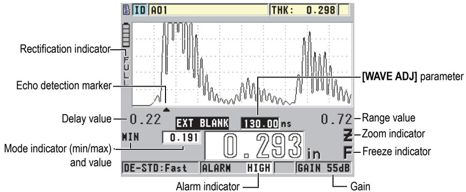
**Figure 3-5 Other elements – Waveform option enabled**
