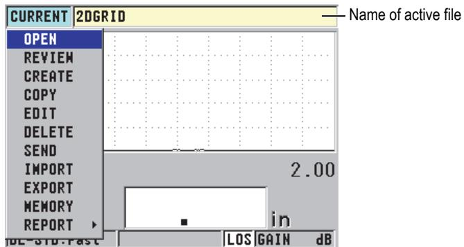
Figure 5-13 The active file name appearing in the ID bar
