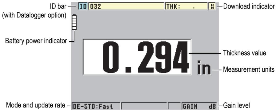
**Figure 3-1 The measurement screen – No waveform enabled**
