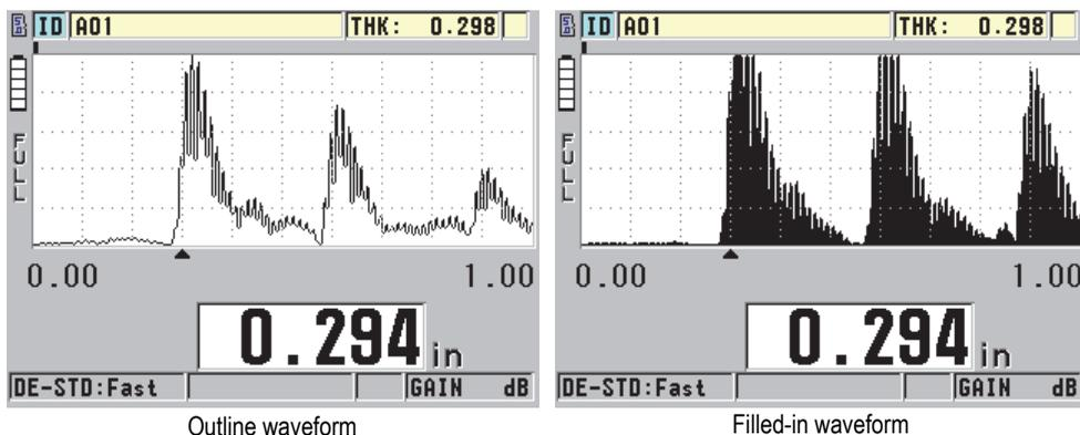
Figure 6-10 Examples of waveform trace modes
