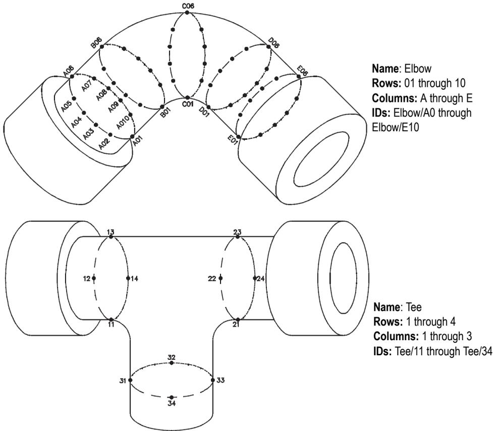
**Figure 6-23 Differently named grid for each part**
