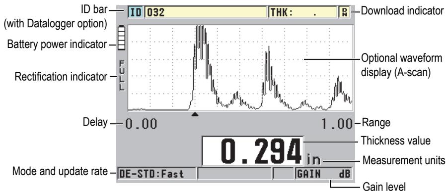
**Figure 3-2 The measurement screen – Waveform option enabled**
