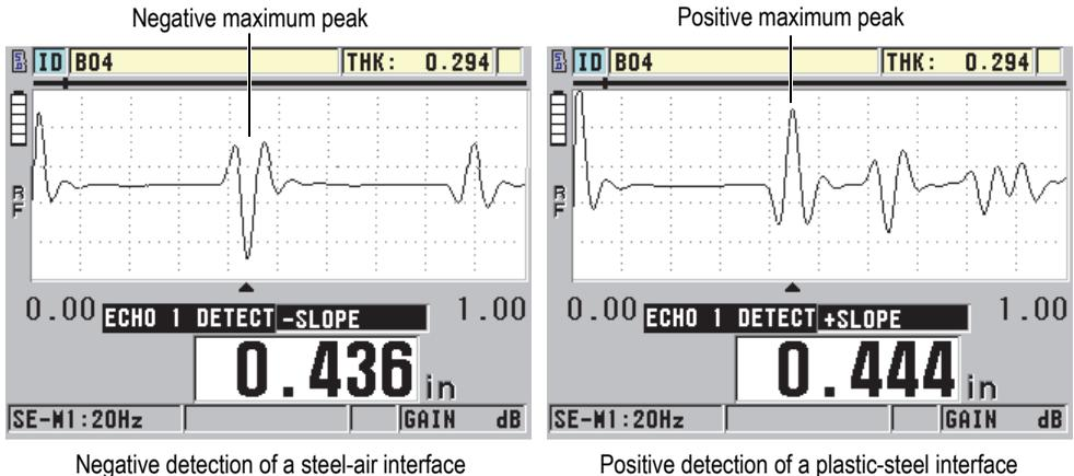
Figure 10-13 Negative and positive echo detection examples
