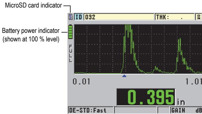
Figure 2-1 The power indicator when using batteries
