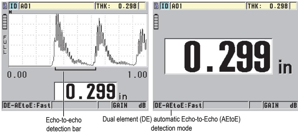
Figure 6-3 Measuring with the automatic Echo-to-Echo detection mode
