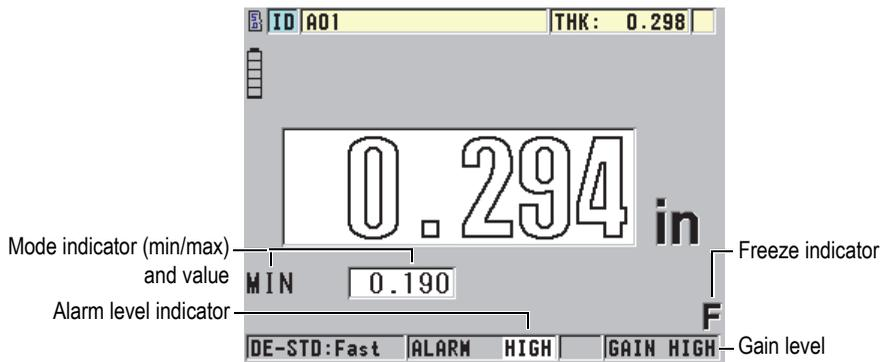
**Figure 3-4 Other elements – No Waveform option enabled**
