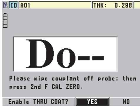
Figure 6-6 Opening the THRU-COAT setup dialog box
