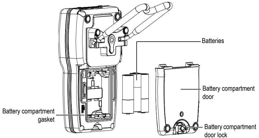
**Figure 2-3 Opening the battery compartment**
