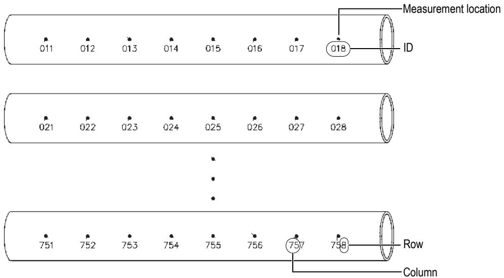
**Figure 6-22 One grid for 75 identical parts**
