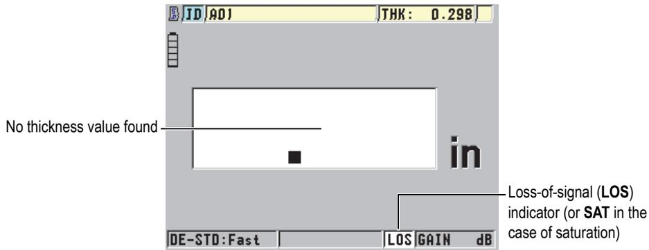
**Figure 3-6 The loss-of-signal (LOS) indicator**
