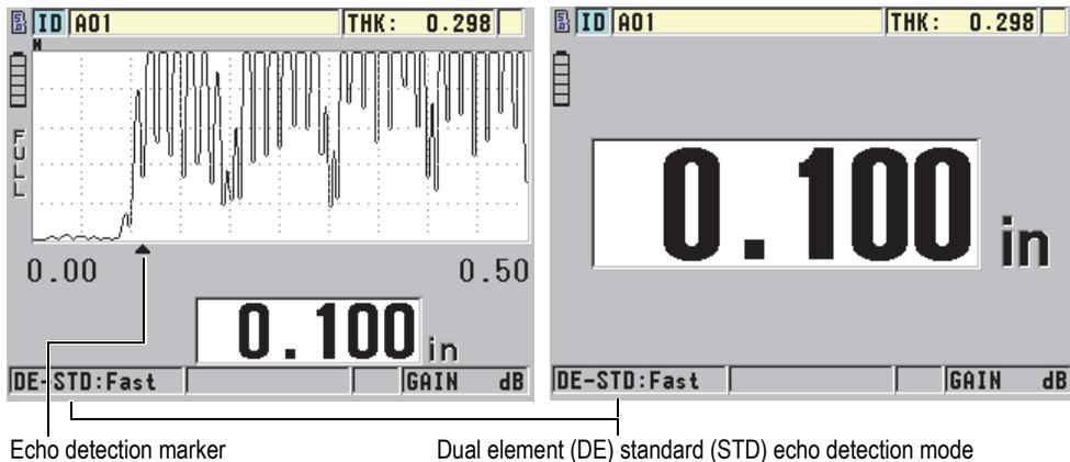
**Figure 6-2 Measuring with the standard echo detection mode**
