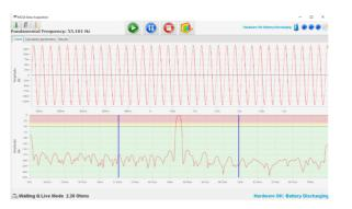
To increase your ability in assessing a machine's rotor/ mechanical performance, the HVPD Kronos® Spot Tester has an add-on Motor Current Signature Analysis (MCSA) feature - non-intrusive, on-line test technique, used to assess the rotor condition of motors by analysing the frequency content of the current.
